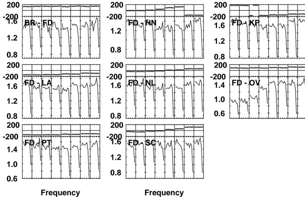
Fig. 1.— POSSM plot of the cross-correlation spectrum of a set of widely spaced IFs in the 4cm band. Multi-band delays are evident in the phase slopes across all the IFs.
