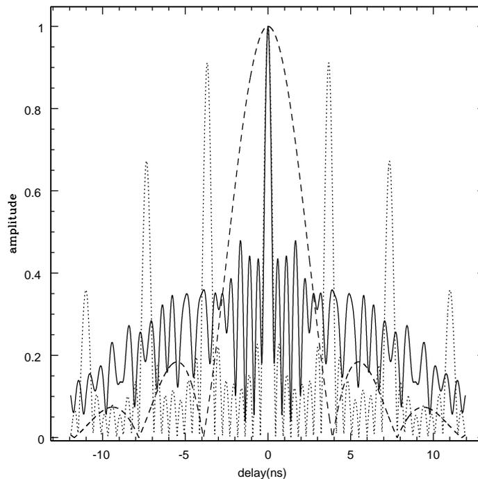
Fig. 2.— Delay function for various IF spacings. Solid line: *Golomb ruler* spacing of 8 IFs across 500 MHz; dashed line: contiguous 64 MHz; and dotted line: 8 IFs evenly spaced across 500 MHz.
