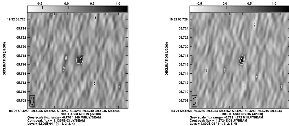
Fig. 6.— Images of same source from the same observation at 8.5 GHz. The image of the left was reduced in the standard phase referencing manner (*i.e.*, with no atmospheric/clock correction), the image on the right was reduced as described in this memo.
