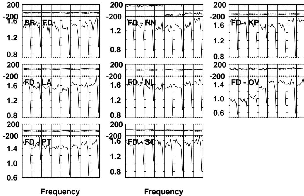
Fig. 5.— POSSM plot of the same scan seen in figure 1 after the tropospheric and clock delays were removed by DELZN.
