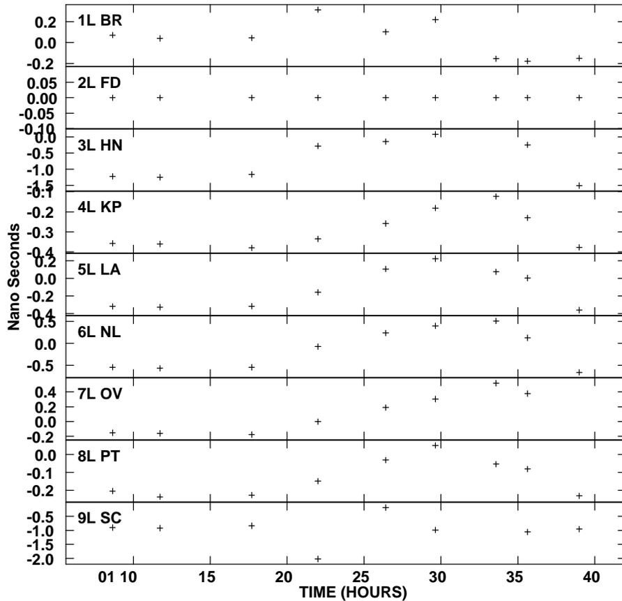
Fig. 3.— SNPLT of MBD versus time. The MBD were found by the *AIPS* task MBDLY. Note that most of the delays are significantly less than 1 nanosecond. FD has zero delay because it is the reference antenna.
