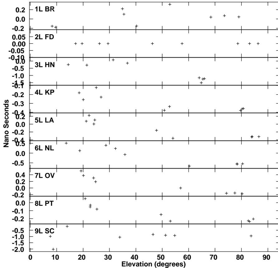
Fig. 4.— SNPLT of MBD versus source elevation. The MBDs were found by the *AIPS* task MBDLY. FD has zero delay because it is the reference antenna.
