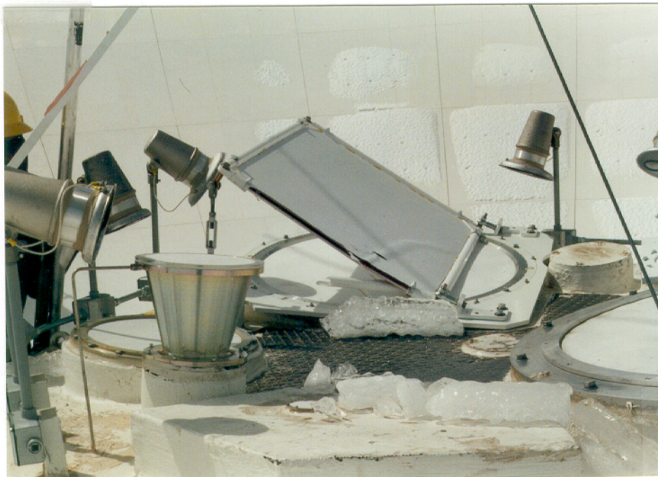
Figure 20. Ice damage to the dichroic plate during the winter storm of 14mar93.
