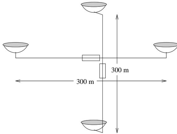
Figure 6: Option 4: Placing the interferometers in different orientations provides information on anisotropic turbulence. However, other interferometer arrays such as the VLA can study this effect already. Typically, phase fluctuations on baselines perpendicular to the wind agree with fluctuations on parallel baselines to 20 or 30%.
