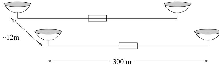
Figure 7: Option 5: Placing the antennas for the interferometer pairs 10-20 m apart would provide a test of the paired antenna calibration method. The orientation of the vector between the paired antennas is not specified, but if the interferometers were colinear parallel to the prevailing wind direction, we could also monitor evolution of the turbulence on short scales. At this point, no array is seriously considering paired *antenna* calibration.
