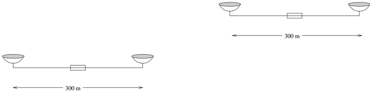
Figure 5: Option 3: Two 300 m baselines monitor the turbulence on different parts of the site. A comparison between the NRAO Chajnantor interferometer and the NRO interferometer 10 km distant at Pampa la Bola has shown that the phase stability can vary by a factor of 5-10. Placing the second interferometer 1-3 km from the existing one on the Chajnantor site would provide interesting data.
