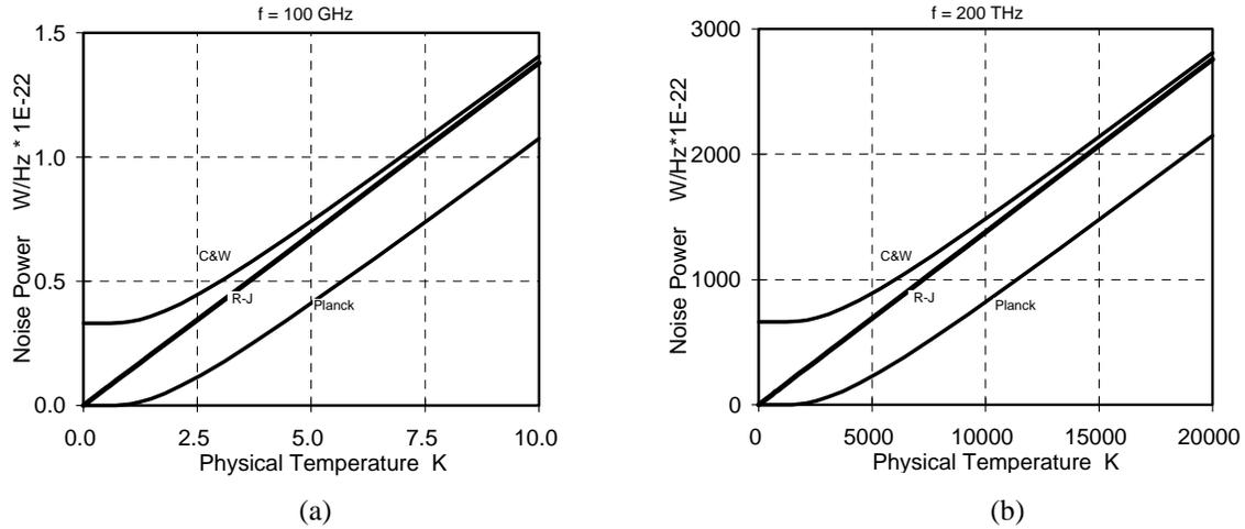
**Fig. 1. Noise power density vs physical temperature for a resistor, computed at (a) 100 GHz and (b) 200 THz ( $\lambda = 1.5 \mu\text{m}$ ) according to the Rayleigh-Jeans, Planck, and Callen & Welton laws.**
