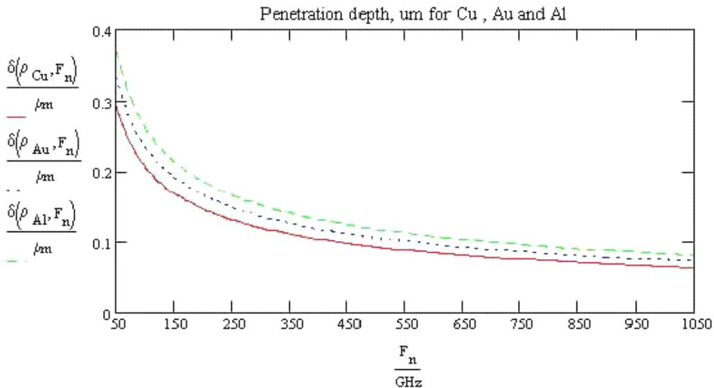
**Figure 5** Penetration depth [mm] for copper (red), aluminum (blue) and gold (green) as a function of frequency.
