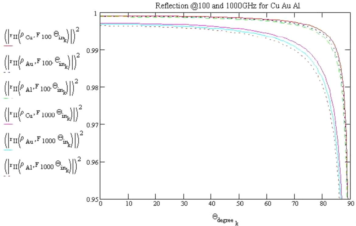
**Figure 3** The reflection coefficient, for the metal mirror made from aluminum, copper and gold vs. angle of incidence. The calculation made for the two frequencies, 100 and 1000 GHz. The two families of the curves present the reflection for *parallel* polarization, the lower curves? family for 1000 GHz.
