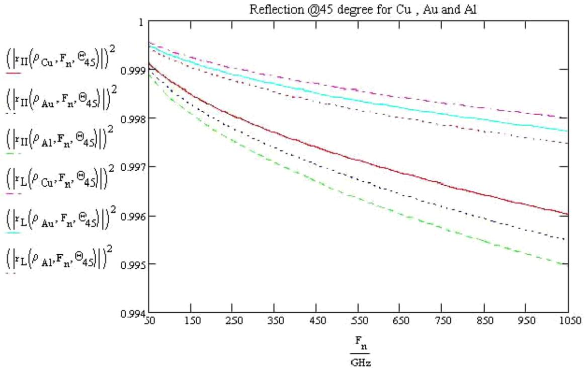
**Figure 1** Reflection of the metal mirror made from aluminum, copper and gold. RF radiation comes at the angle of incidence  $45^\circ$ , the two families of the curves present the reflection for the metals for parallel (II) (lower curves family) and the normal (L) polarization. Curves color coding is according to the legend to the left.
