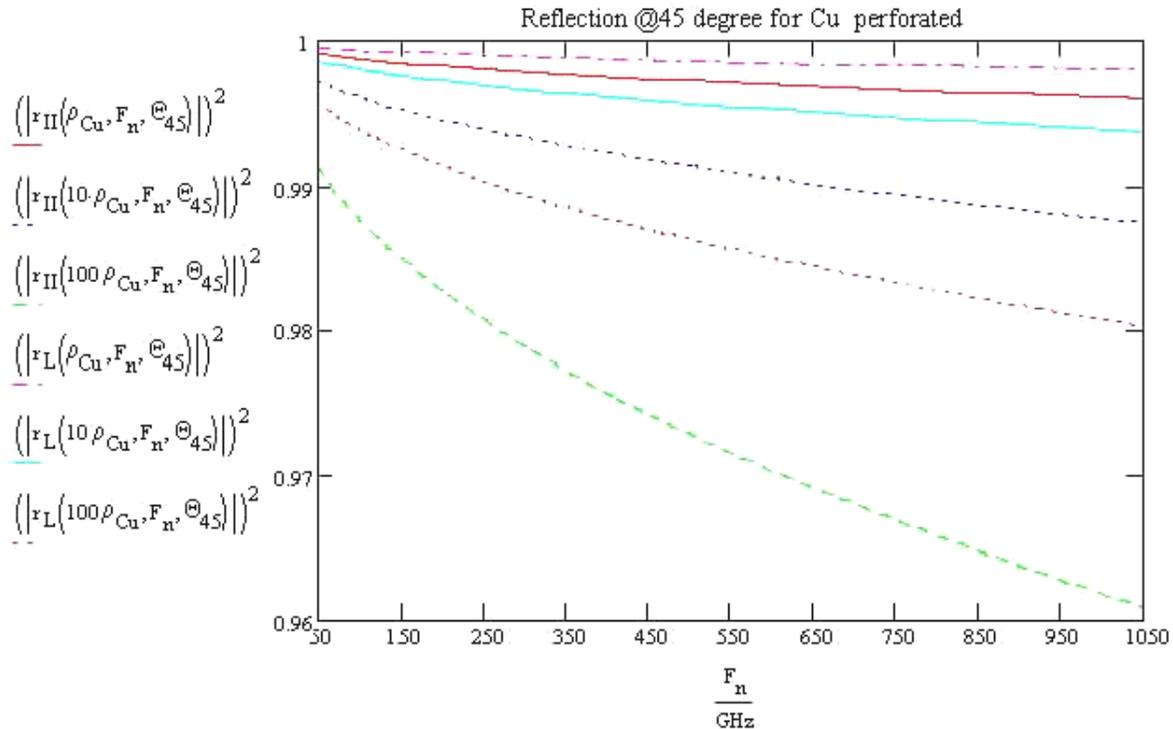
**Figure 6** Modeled reflectivity of the Cu perforated surface. The solid red curve and the dash-dot magenta curve present reflectivity of the solid Cu metal surface for parallel (II, the even curves, from the top to the bottom) and normal polarization (L). Incidence angle is  $45^\circ$ , the ratios of the of the perforated/metal areas per unit of the reflector area are 10 and 100 (color coding at the left).
