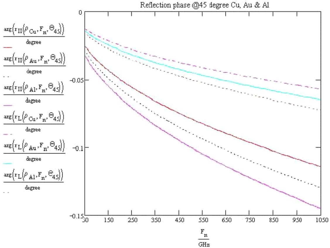
**Figure 2** Phase of the reflection coefficient, angle degrees, for the metal mirror made from aluminum, copper and gold. RF radiation comes at the angle of incidence  $45^\circ$ , the two families of the curves present the reflection phase for the metals for *parallel* (lower curves family) and the *normal* polarization. Curves color coding is according to the legend to the left.
