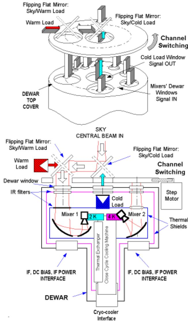
**Figure 7** Suggested LSA/MMA receiver layout. Each mixer in the drawing represents dual-polarization mixer unit.
