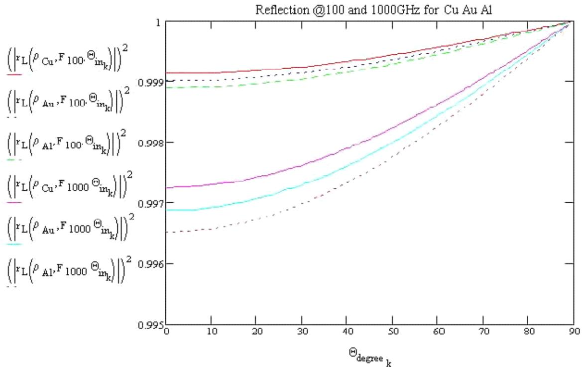
**Figure 4** The reflection coefficient, for the metal mirror made from aluminum, copper and gold vs. angle of incidence. The calculation made for the two frequencies, 100 and 1000 GHz. The two families of the curves present the reflection for *normal* polarization, the lower curves? family for 1000 GHz.
