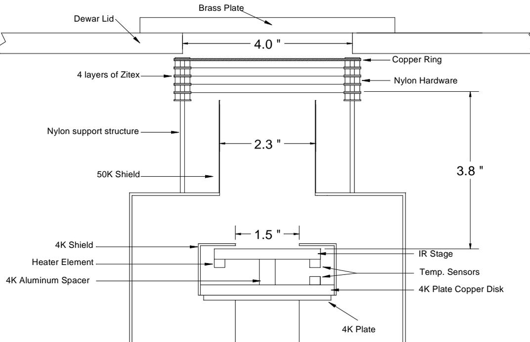
Figure 1. Experimental Setup for Floating IR Shield Test
