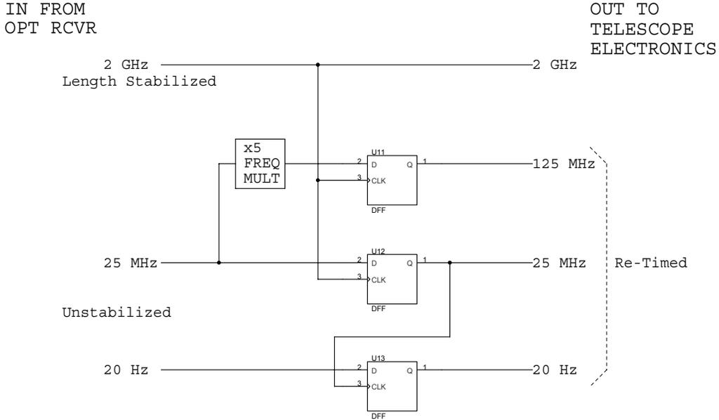
Figure 2: Ambiguity resolution circuit.
