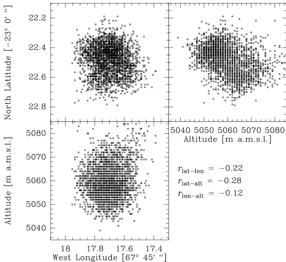
Figure 4: Positions measured after discontinuation of SA and linear cross correlation coefficients. Note scale difference between latitude-longitude and altitude;  $0.1''$  corresponds to 3.1 m.
