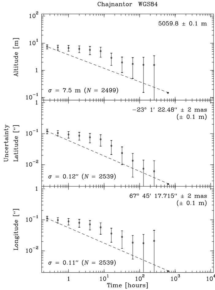
Figure 6: Variance in the mean positions for successively longer sets of measurements after SA was discontinued. The error bars illustrate the sampling uncertainty for a normal distribution,  $\sigma_\sigma/\sigma = (2/(N - 1))^{1/4}$  (Bailey 1971). The dashed lines show the decrease with  $N^{0.5}$  expected for sequentially uncorrelated data.
