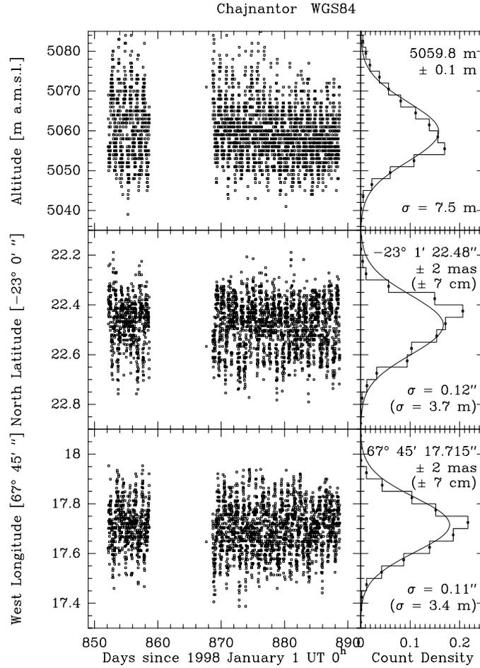
Figure 3: Measured positions of the NRAO equipment container on Chajnantor, Chile, after 2000 May 2 UT 4:00, when SA was discontinued. In the right panels, the histograms show the actual distribution of the measured positions and the curves are normal (Gaussian) distributions for the parameters derived from the data. Note scale difference between latitude-longitude and altitude and between Figures 1 and 3.
