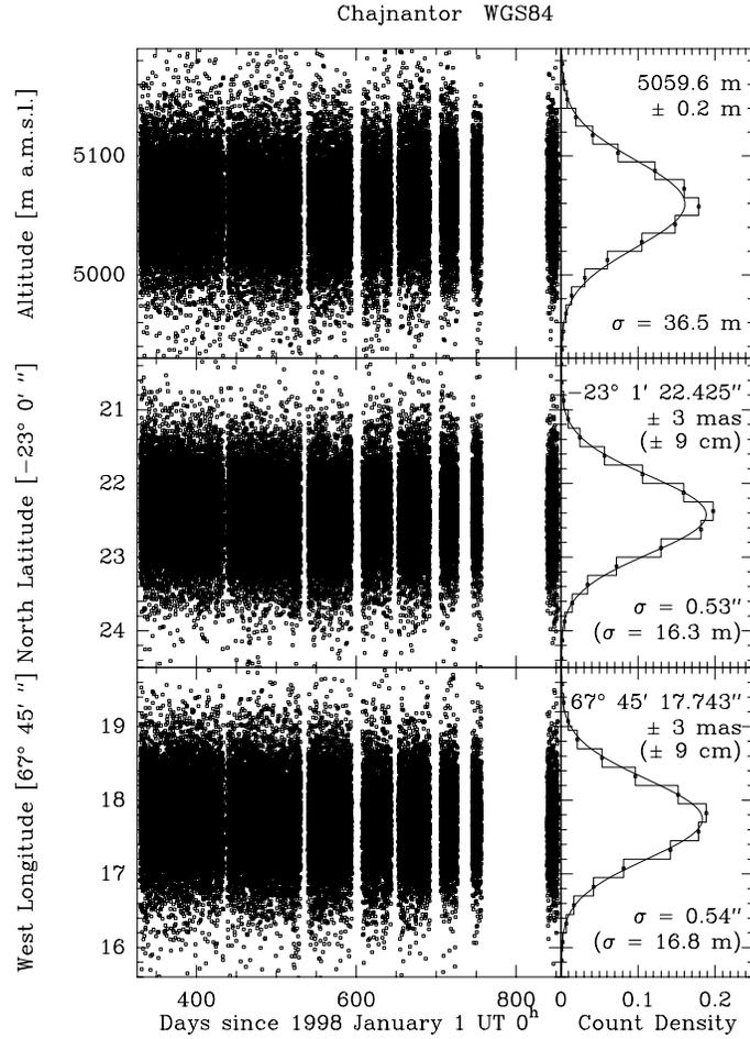
Figure 1: Measured positions of the NRAO equipment container on Chajnantor, Chile, from 1998 November 26 UT 19:30 until 2000 May 2 UT 4:00, when SA was active. In the right panels, the histograms show the actual distribution of the measured positions and the curves are normal (Gaussian) distributions for the parameters derived from the data. Note scale differences between latitude-longitude and altitude and between Figures 1 and 3.
