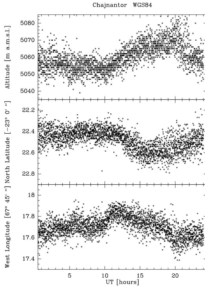
Figure 5: Diurnal variation of positions measured after discontinuation of SA. Note scale difference between latitude-longitude and altitude;  $0.1''$  corresponds to 3.1 m.
