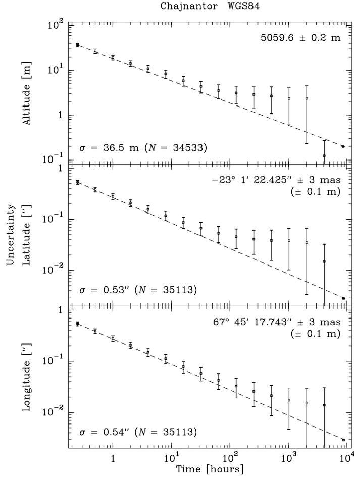
Figure 2: Variance in the mean positions for successively longer sets of measurements when SA was active. The error bars illustrate the sampling uncertainty for a normal distribution,  $\sigma_\sigma/\sigma = (2/(N - 1))^{1/4}$  (Bailey 1971). The dashed lines show the decrease with  $N^{0.5}$  expected for sequentially uncorrelated data.
