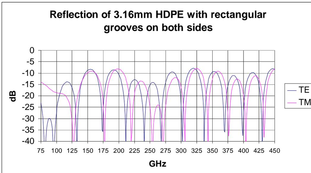
**Figure 6** Calculated reflection.
