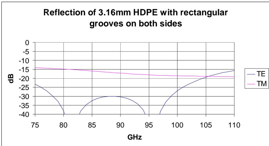
**Figure 8** Calculated reflection.
