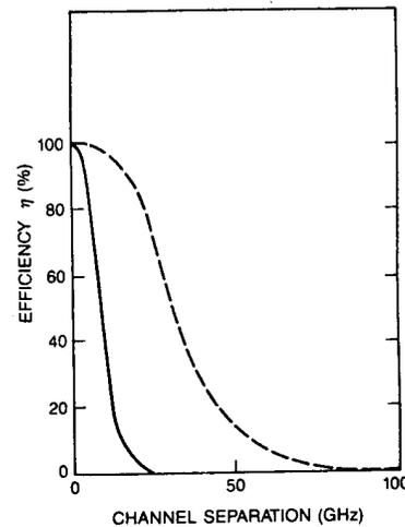
**Fig H.1 Four Wave Mixing efficiency as a function of channel separation at 1.55 $\mu$ m. The solid curve represents Single Mode Fibre (SMF) with dispersion = 16ps/nm · km. The dashed curve is for dispersion-shifted fibre (DSF) with dispersion of 1ps/nm · km.**
