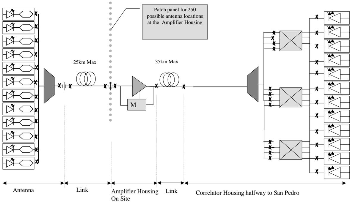
The power budget below shows that this link design is possible using only one amplifier. Since there is not a great margin left in the power budget this strategy requires further, practical investigation to ensure it is a robust design which could be practically implemented.
