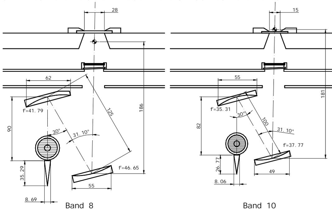
Figure 6. Band 8 and 10 layouts. The LO is injected at the polarizing grid.
