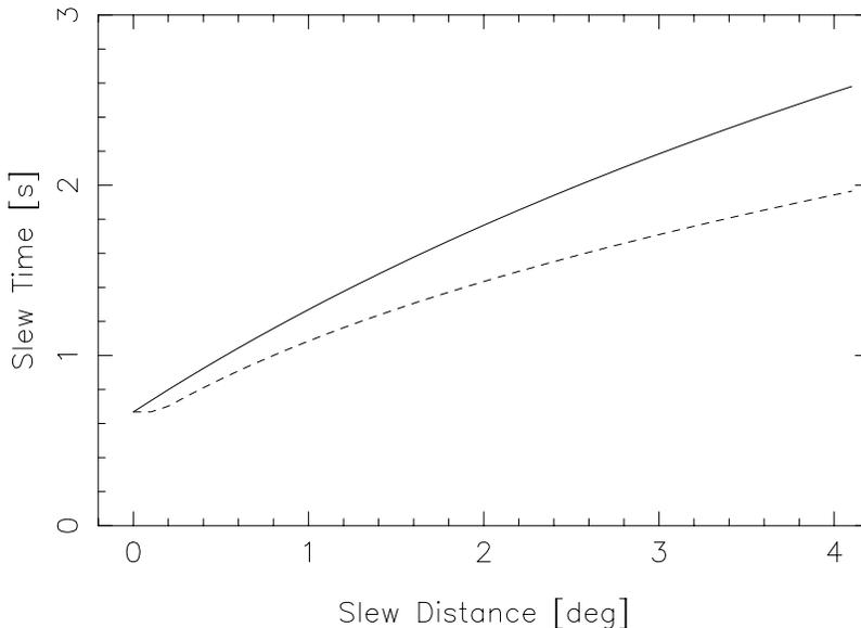
Figure 1: Modeled slew times for azimuth and elevation slews.
