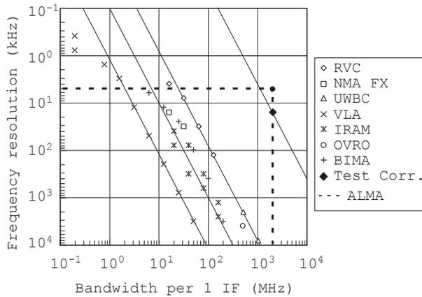
**Fig. 1.** Specifications of the frequency-resolution and bandwidth for several correlators. RVC is reported by Iguchi et al. (2000), NMA-FX by Shibata (1996), UWBC by Okumura et al. (2000), and the test correlator by Iguchi et al. (2002). Correlators of the VLA, IRAM, OVRO, and BIMA are also shown based on their Web pages or status reports. The scientific requirements for the ALMA are shown by the dashed lines.
