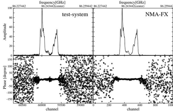
**Fig. 5.** Comparison of the SiO fringe spectra with a 32-MHz bandwidth between the test correlator and the NMA-FX correlator. The upper panels show the amplitude, while the lower panels show the phase. The amplitude is normalized in the same manner as in figure 3
