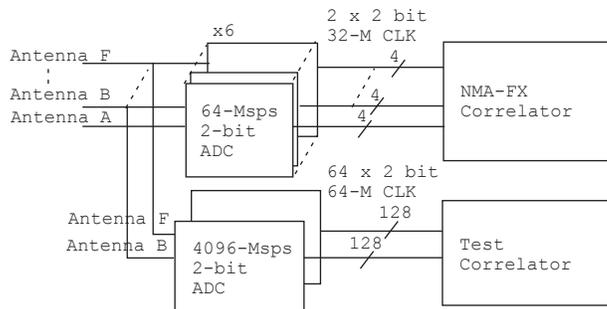
**Fig. 2.** Block diagram of the observational setup.
