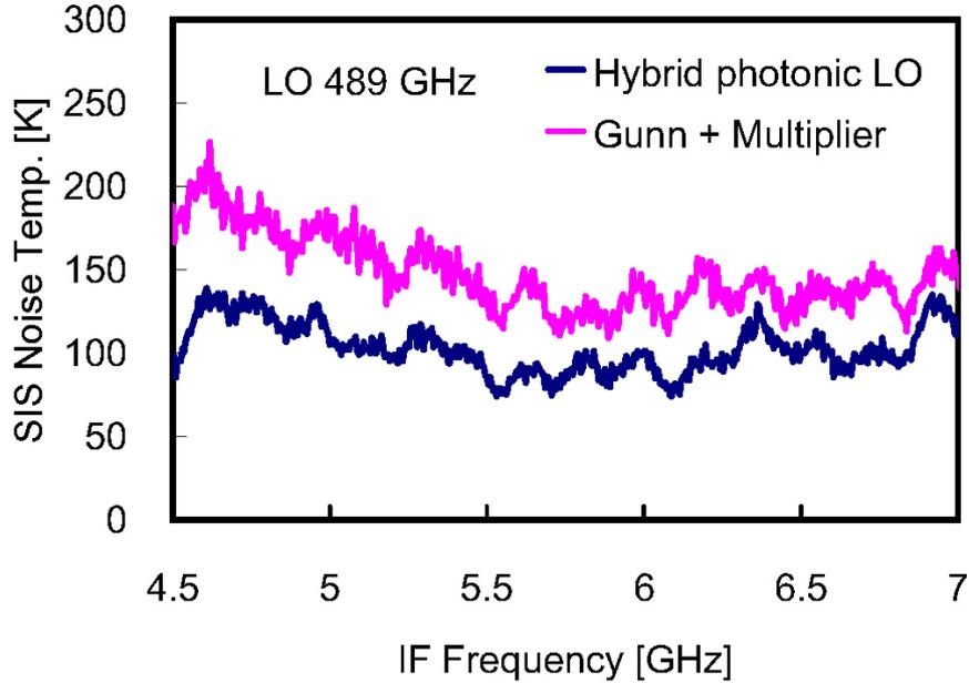
Figure 6: Noise temperatures of an SIS receiver pumped by a hybrid photonic LO and a Gunn LO with respect to IF frequency at an LO frequency of 489 GHz. The LO power for the SIS receiver by a Gunn LO is not optimum. Because the temperature scale was calculated from the Rayleigh Jeans approximation, the temperature is lower by 10 K than that from the Planck formula.
