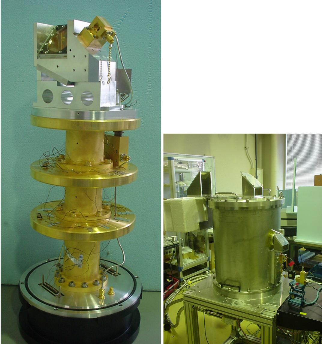
Figure 2: The left picture shows the engineering model of band 8 cartridge and the right shows a cartridge test cryostat.
