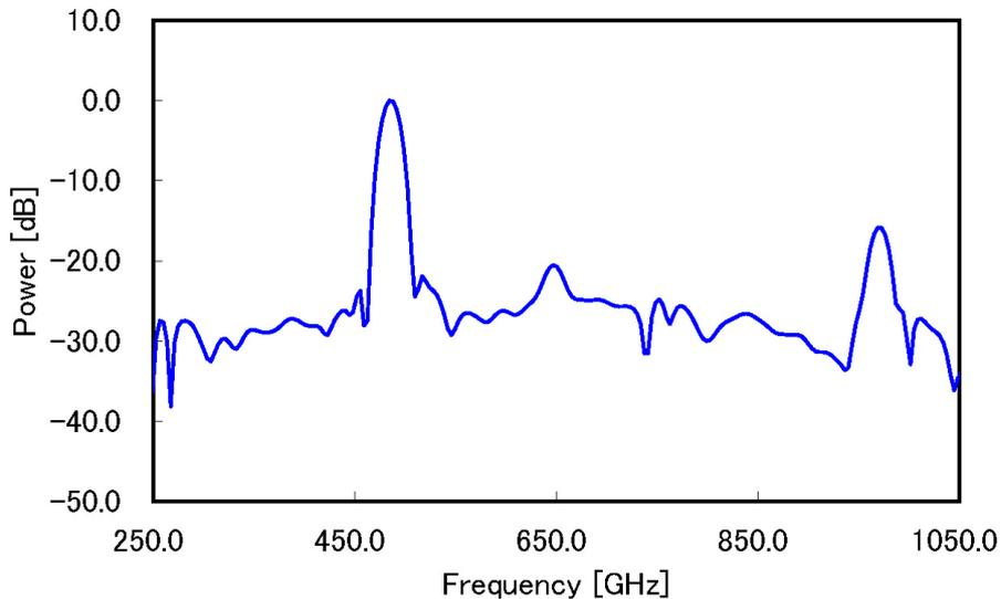
Figure 4: Fourier transform spectrometer (FTS) spectra for a multiplier manufactured by Radiometer Physics (RPG). The RPG multiplier composed of a doubler and a tripler is driven by a Gunn oscillator at a frequency of 80.8 GHz. The dual-mode horn is attached for the RPG multiplier.
