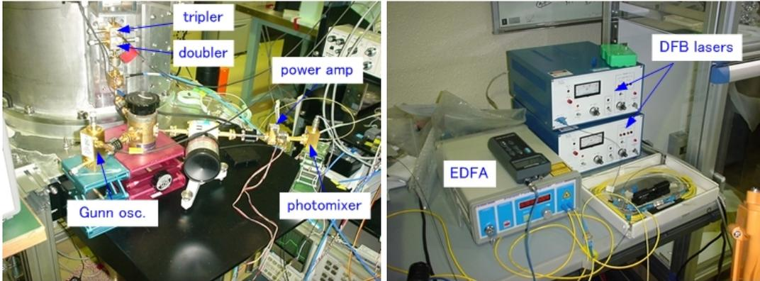
Figure 3: The left picture shows photonic and Gunn local oscillators and the right picture shows DFB lasers.
