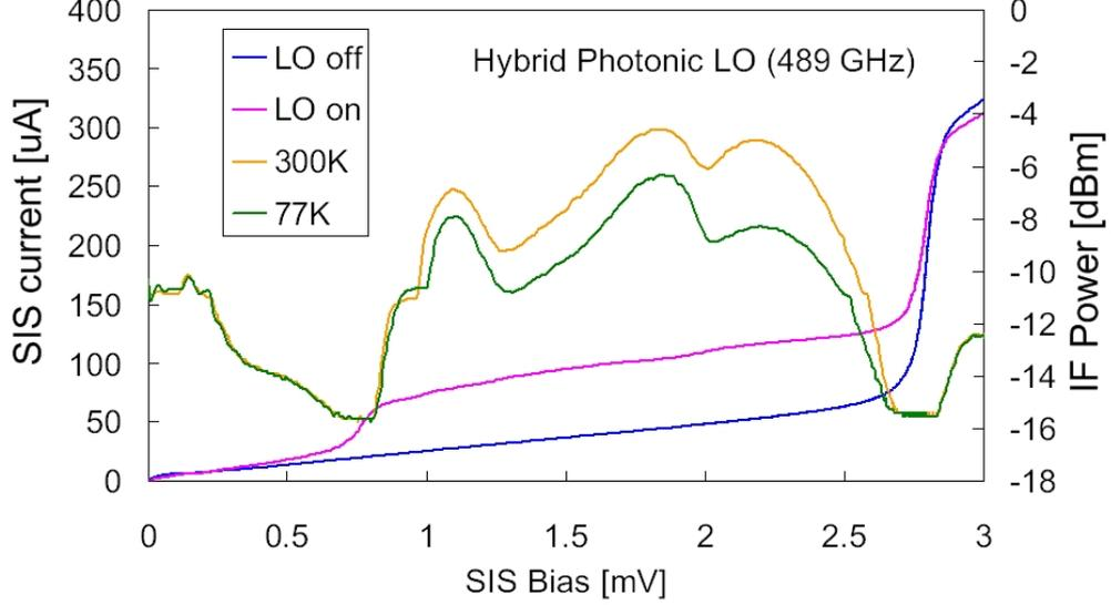
Figure 5: SIS mixer’s I-V and IF-power bias-voltage curves pumped by a hybrid photonic LO at a frequency of 489 GHz. At a bias voltage of 2.2 mV, the Y-factor was 3.2 dB, which corresponds to a noise temperature of 135 K from the Plank formula. The dips at 1.0 and 2.0 mV on the IF-power curve are Shapiro steps ( $hf/2e = 1.008$  mV).
