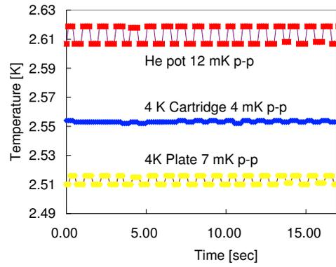
Figure 9: The temperature variation on the 4 K stage and plate in 20 seconds. The ripple is associated with the cold head displacement of 3 stage GM cryocooler.
