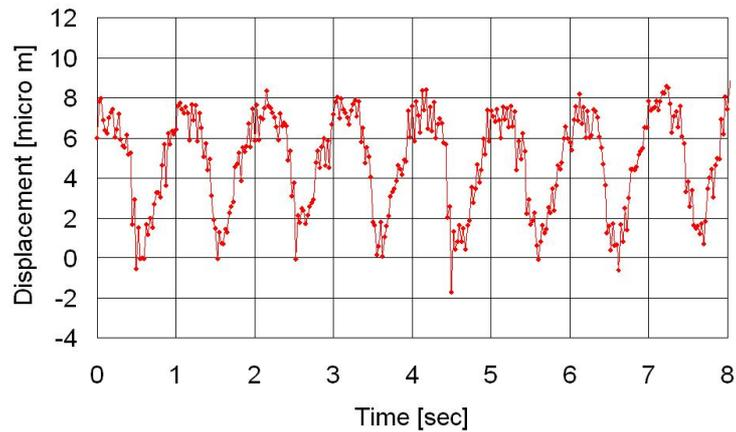
Figure 12: The horizontal vibration on the 4 K stage of the cartridge.
