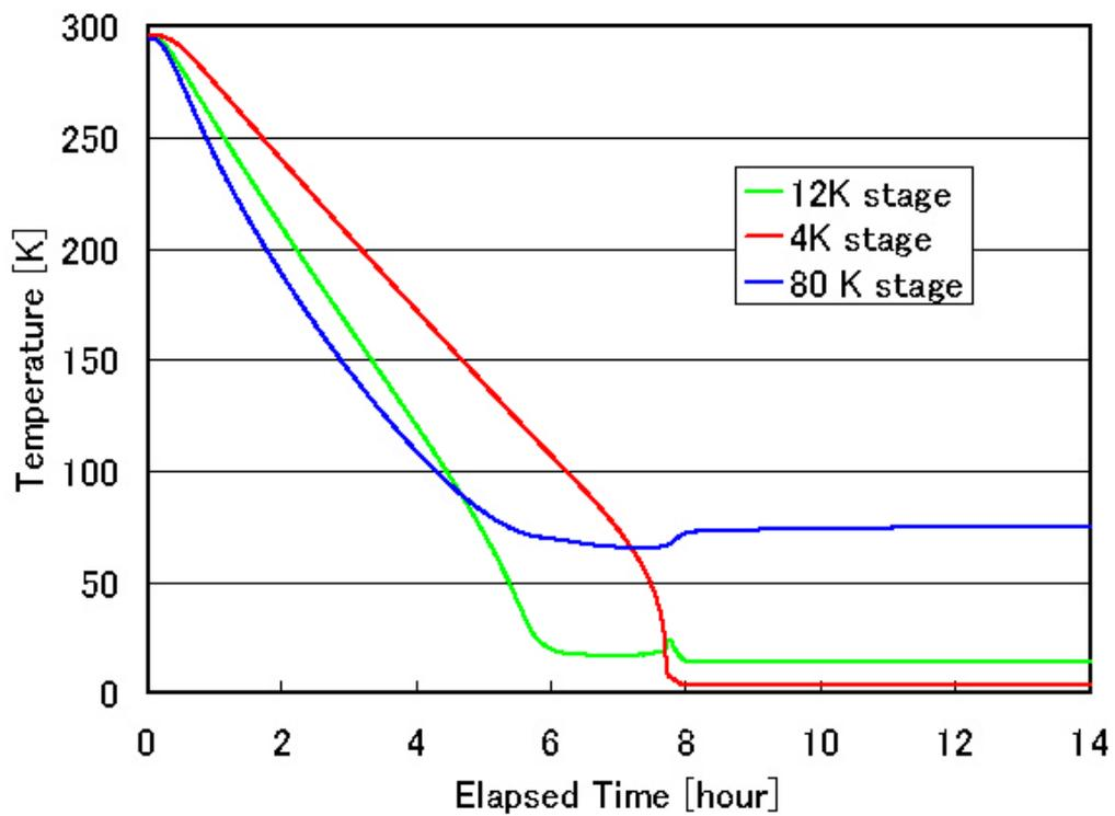
Figure 8: Cooling time of a cartridge-type cryostat.
