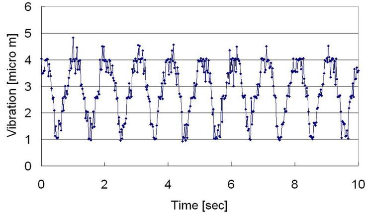
Figure 11: The vertical vibration on the 4 K stage of the cartridge.
