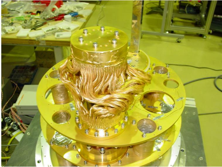
Figure 5: A coldhead interface to reduce the mechanical vibration
