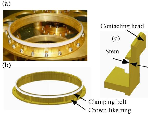
Figure 4: (a) A photograph of the thermal link. (b) Cross-sectional view of the thermal link. The link is composed of a crown-like ring made of oxygen free copper and clamp belt made of nylon. The crown-like rings divided to 120 pieces. (c) Up side view of the thermal link.
