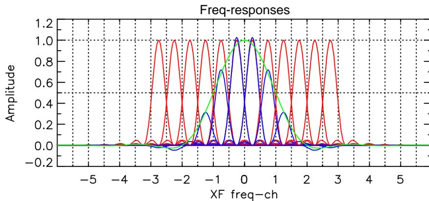
**Figure 3 Frequency responses of FX and XF correlators**
