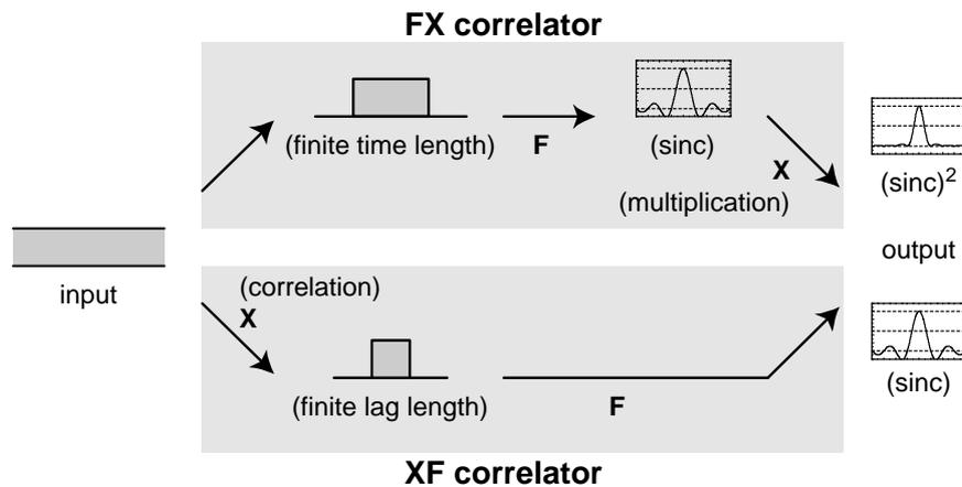
**Figure 1 Calculation order of “F” and “X” in FX and XF correlators**
