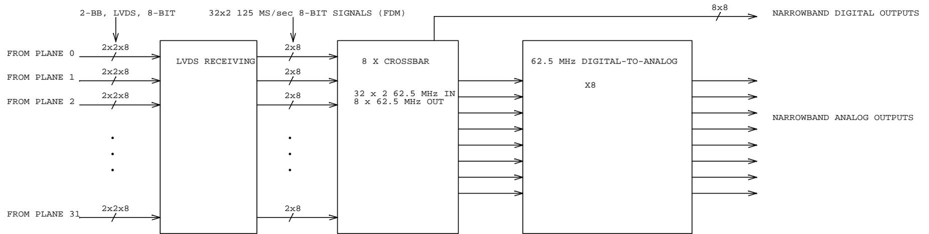
FIGURE 1 BLOCK DIAGRAM OF PHASED SUMMATION LOGIC (FREQUENCY DIVISION MODE)
