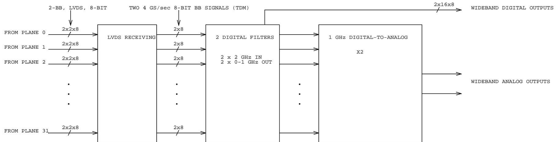
FIGURE 2 BLOCK DIAGRAM OF PHASED SUMMATION LOGIC (TIME DIVISION MODE)
