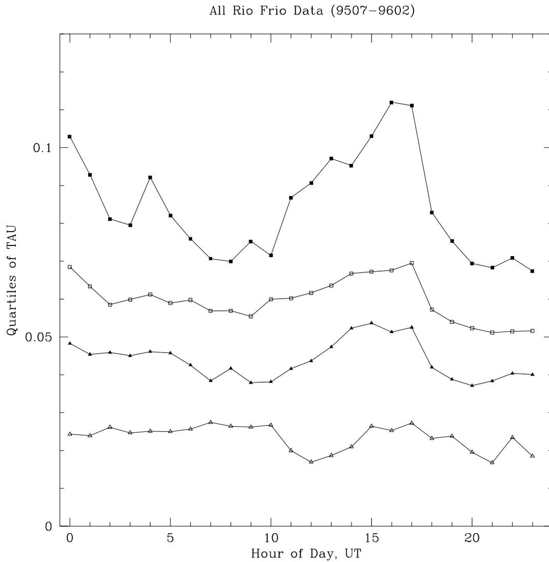
Figure 5: Diurnal fluctuations of the opacity using all radiometer data from Rio Frio. The variations are very small, and only during the worst conditions do day time opacities show a marked increase over the night time values.
