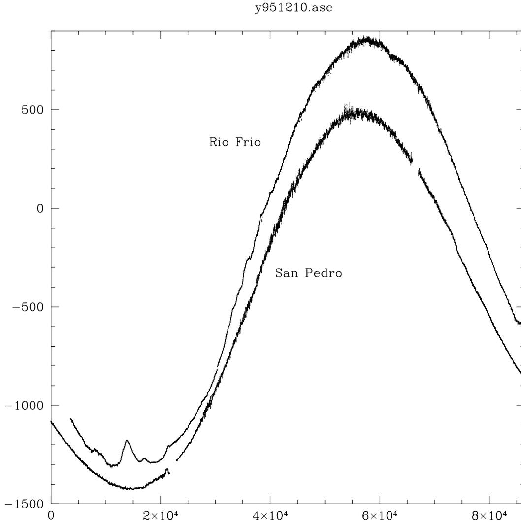
Figure 6: The raw phase data from Rio Frio (bumpy line) and Chajnantor (line with two small breaks) for one day indicates that there are some medium time scale (10-60 minutes) phase excursions in the Rio Frio data. These phase excursions do not appear to be correlated with any measured weather data.
