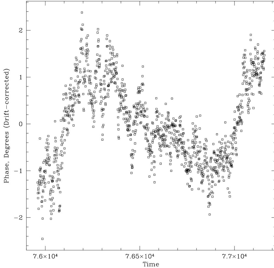
Figure 7: We zoom in to take a close look at one of the anomalous phase excursions after a quadratic trend has been removed from a 20 minute phase time series. The dominant “z” shape is probably instrumental rather than atmospheric, and will leave some residual effect on 10 minute phase time series.
