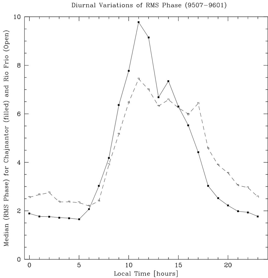
Figure 14: Diurnal variation of the median rms phase on the Rio Frio (solid lines, filled boxes) and Chajnantor (dashed lines, empty boxes) sites. This plot only includes data when the radio seeing monitors at both sites were functional.
