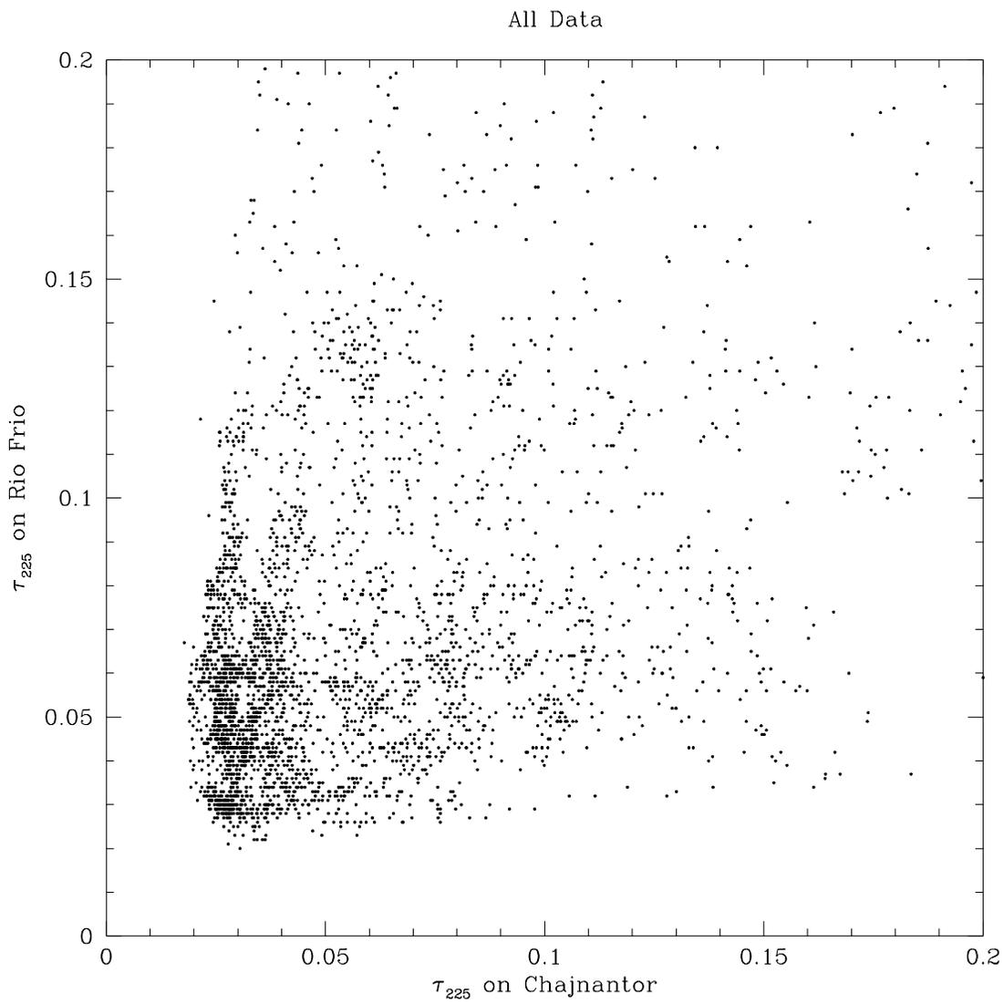
Figure 3: Rio Frio opacity plotted against Chajnantor opacity. This plot only includes data when the radiometers at both sites were functional.
