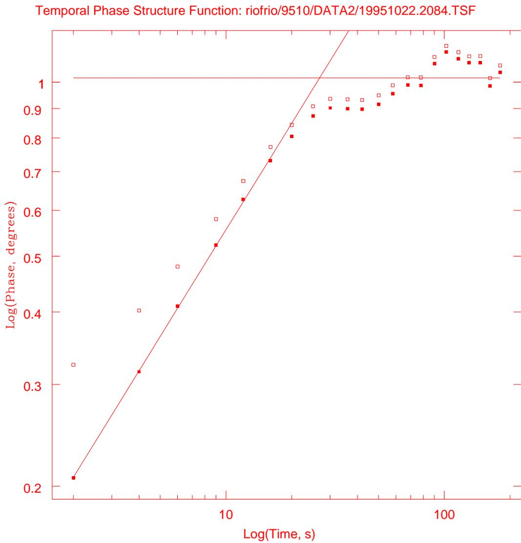
Figure 8: The calculated temporal phase structure function at a time of good phase stability (open boxes) and the structure function after removing the 0.25 degree noise term.
