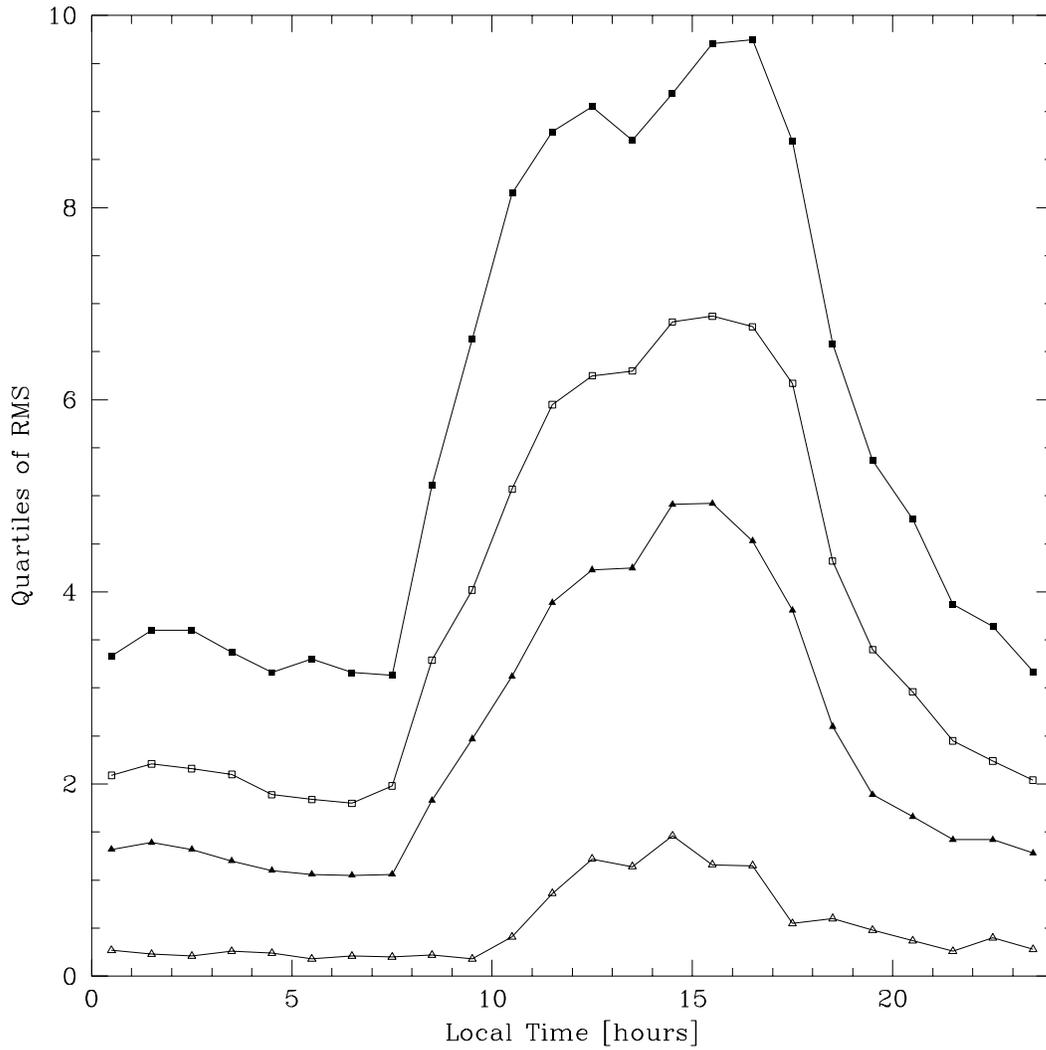
Figure 9: Diurnal variations of the rms phase in degrees over 600 s using all Rio Frio phase stability data. The lowest curve is for the best phase conditions observed, and the other three curves are for the first, second, and third quartiles rms phases.
