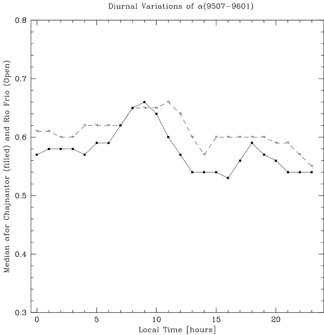
Figure 15: Diurnal variation of the median structure function exponent on the Rio Frio (solid lines, filled boxes) and Chajnantor (dashed lines, empty boxes) sites. This plot only includes data when the radio seeing monitors at both sites were functional.
