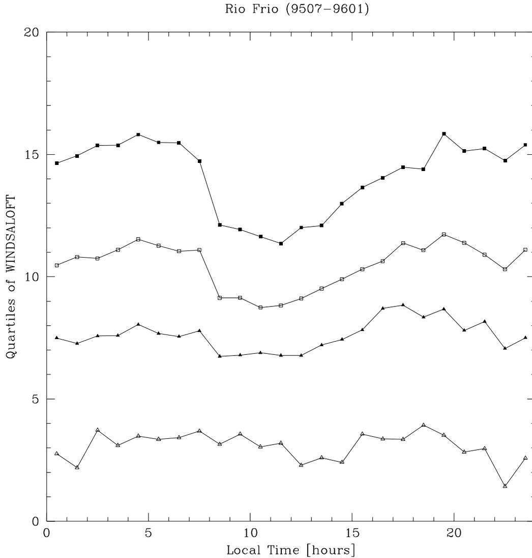
Figure 12: Diurnal variations in the speed of the turbulent water vapor above the interferometer. The lowest calculated speed of the “wind aloft” in m/s, followed by the first, second, and third quartile values are shown for all phase data from the Rio Frio site.
