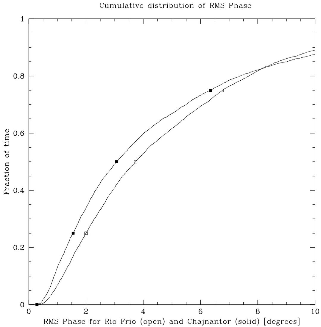
Figure 13: Cumulative distribution of the rms phase at the Rio Frio and Chajnantor sites. This plot only includes data when the radio seeing monitors at both sites were functional.
