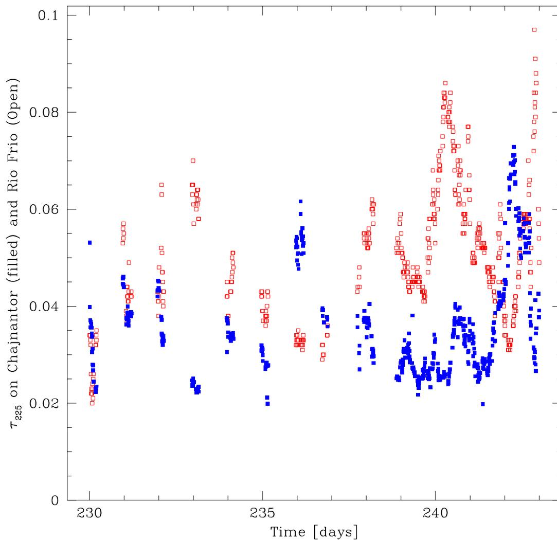
Figure 2: Opacity time series for the two sites. Filled squares are Chajnantor, open squares are Rio Frio, time is in days since 0 hours UT, Jan 1, 1995. This plot only includes data when the radiometers at both sites were functional.
