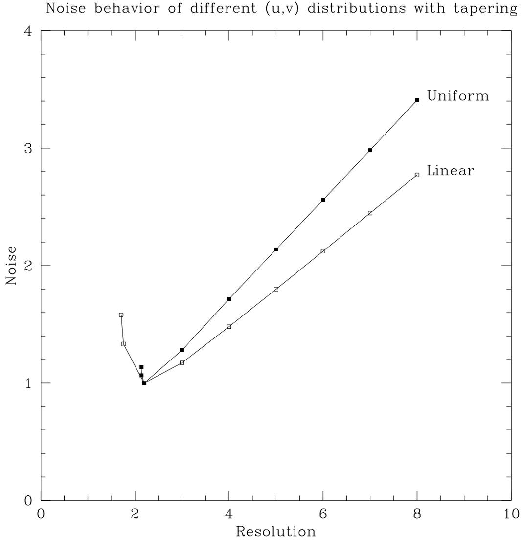
Figure 3: How does point source sensitivity degrade as we taper the Fourier plane coverage? We plot the point source sensitivity, normalized to full array sensitivity, as a function of resolution for uniform and linearly decreasing Fourier plane distributions. The upraised spurs at the highest resolutions are for robust and uniform weighting.
