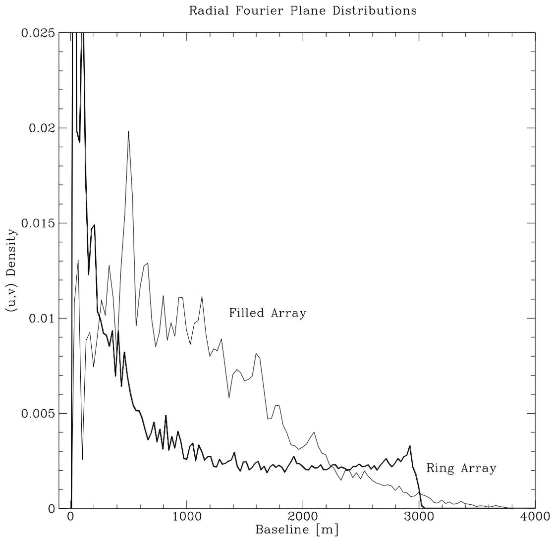
Figure 1: Radial Fourier plane distributions from actual ring and filled circle antenna configurations
