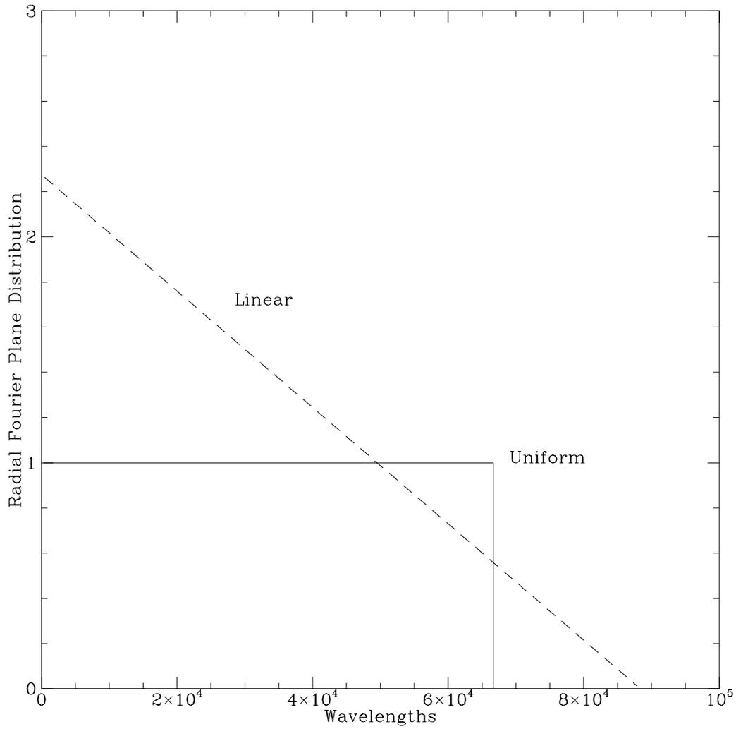
Figure 2: The uniform and centrally condensed (linearly decreasing) Fourier plane distributions used in this study. The radial cuts have been plotted such that the integral over the 2-D Fourier plane is the same for both distributions. Just arguing from geometry, trading a little bit of baseline density in the expansive outer part of the plane buys us a lot of baseline density in the cozy inner plane.
