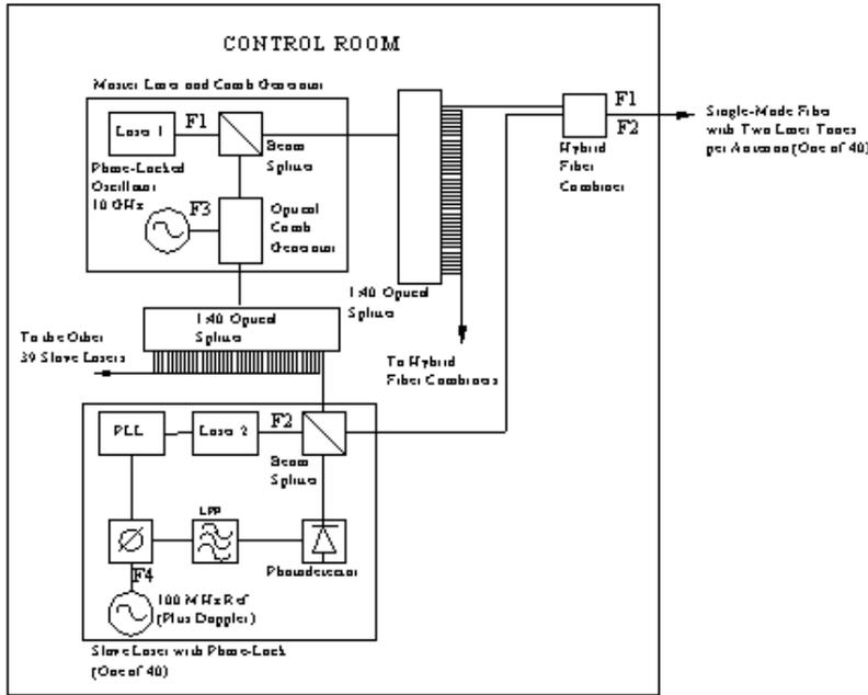
Figure 1 - Laser heterodyne system with optical phase locked loop
