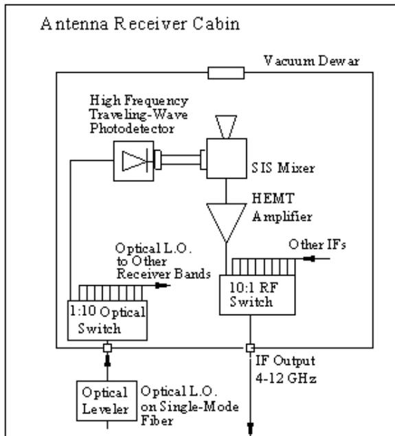
Figure 2 - Photonic LO detection scheme, at receiver
