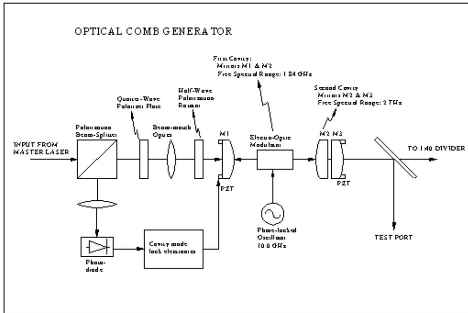
**Figure 4** - Optical Comb Generator - Detailed View
