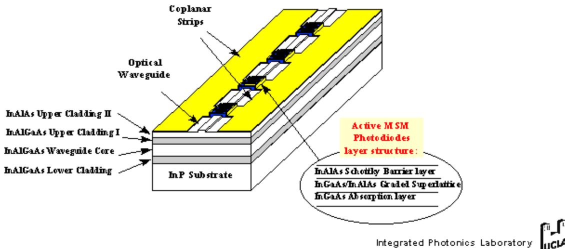
**Figure 3** - Schematic of Long Wavelength Velocity-Matched Distributed Photodetector (VMDP)
