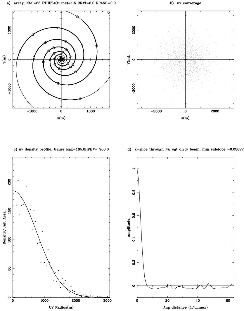
Figure 3: Simulation of a 36 element MMA-only spiral array with  $DTHETA=1.5$  turns per arm over a ratio of radius  $RRAD = 8$  between the first antenna and last antenna. a) Antenna layout. Circles indicate antenna positions, spiral lines indicate the paths taken by the 'road' and conduits for optical fibres, power cables etc. b) uv coverage. c) UV point density versus uv distance. d) Slice through the natural weighted dirty beam.
