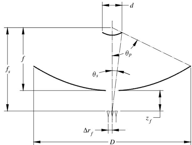
Fig. 1. Parameters for Cassegrain geometry as used in the text. The different receiver bands are separated in the focal plane.
