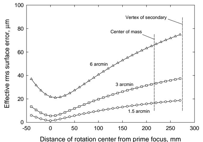
Fig. 3. Effective surface error from aberrations due to rotation of secondary. The curves are labeled with the beam throw on the sky,  $\theta_{sky}$ . The parameters are  $f = 4.8$  m,  $d = 750$  mm, and  $M = 20$ .
