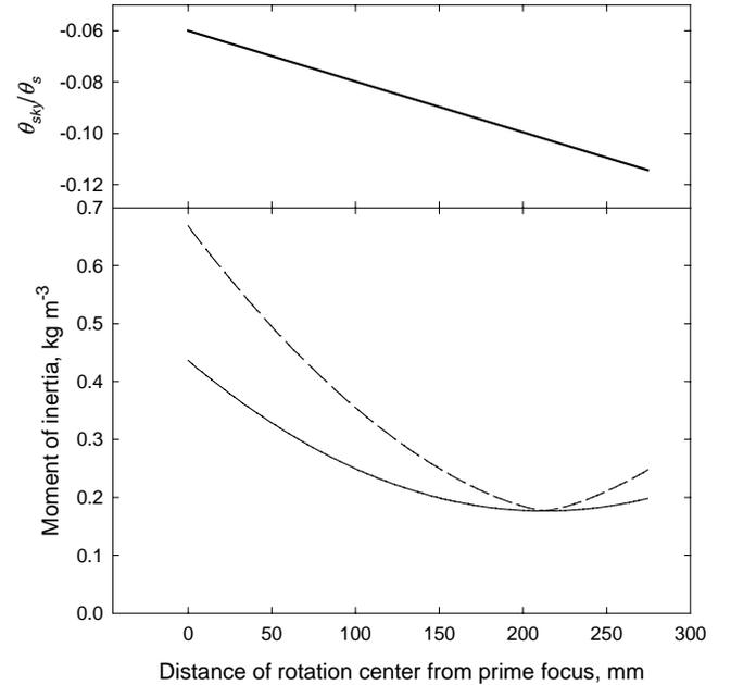
Fig. 5. Total moment of inertia about a point  $z_c$  from the prime focus for the secondary mirror (solid line), and the mirror plus counterbalance (dashed line). The upper graph gives the corresponding factor for the ratio of sky tilt to secondary mirror tilt. Parameters are given in the text.
