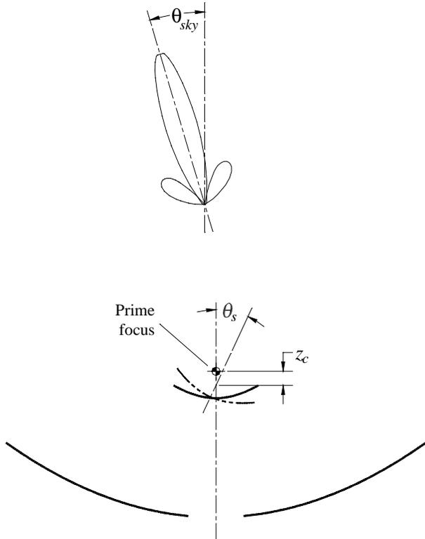
Fig. 2. Geometry and parameters for beamswitching by nutating the secondary mirror.
