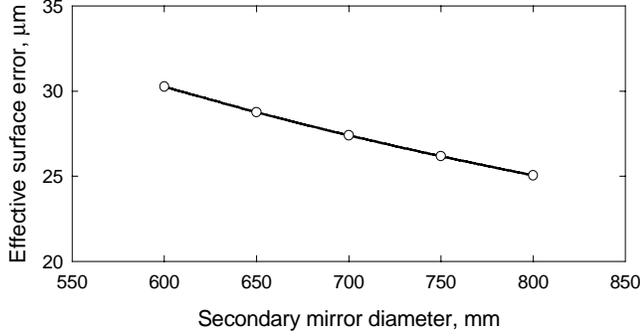
Fig. 4. Dependence on effective surface error on secondary diameter for  $f = 4.8$  m,  $M = 20$ ,  $z_c = 150$  mm,  $\theta_{sky} = 3$  arcmin.
