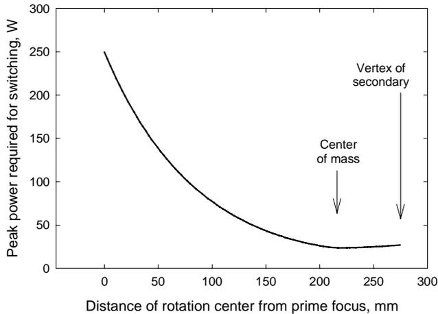
Fig. 6. The peak power needed to drive the secondary for a throw of  $\pm 1.5$  arcmin at 5 Hz rate with a 10% duty-cycle. The average power is a tenth of this.
