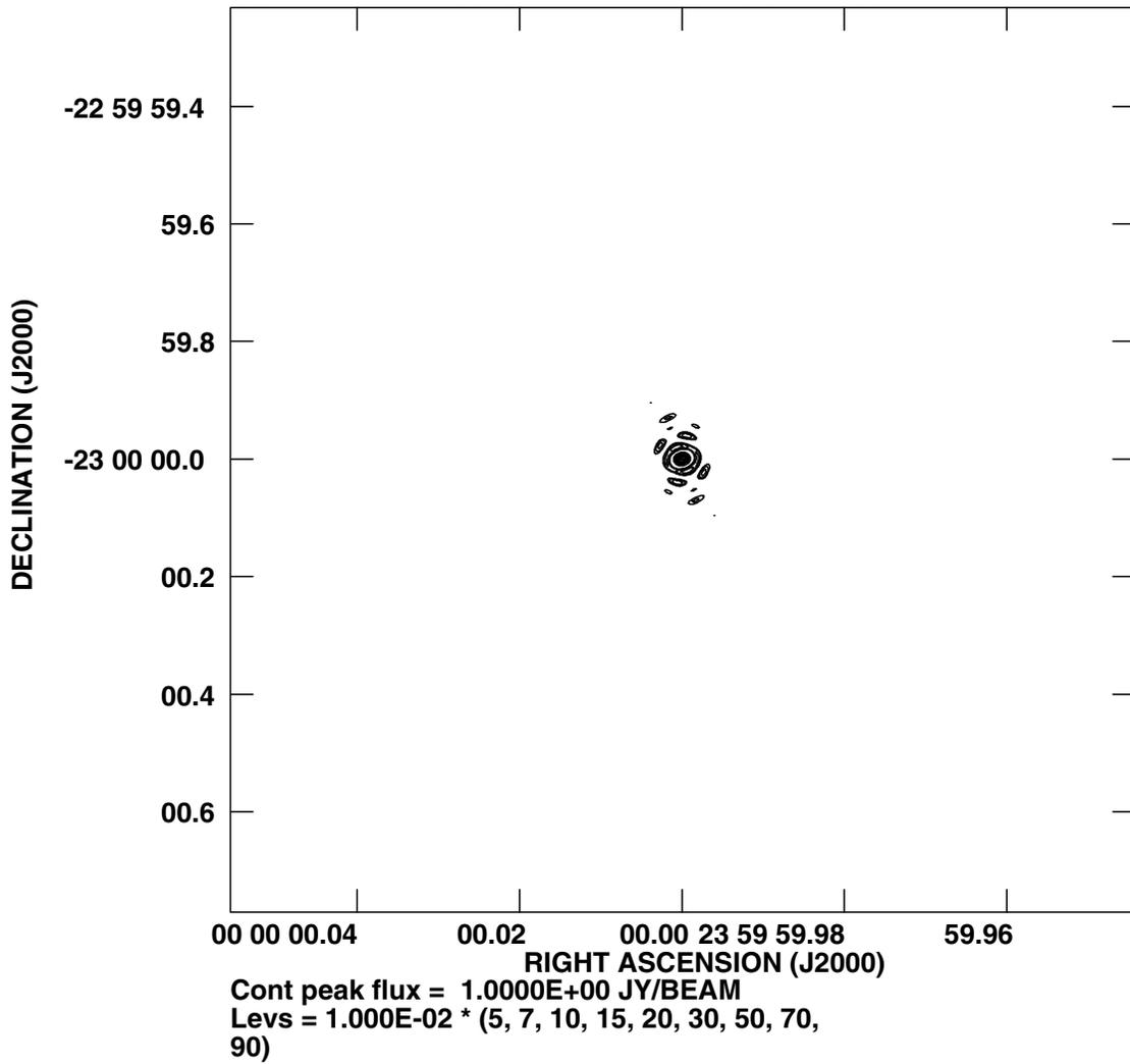
Figure 12: Six hour tracks observations. Beam pattern of the array fitted to the terrain using topography and doughnut constraints. The field ( $512 \times 512$ , cell =  $0.2 \frac{\lambda}{D}$ ,  $\lambda = 1mm$ ) includes far side lobes. The far side lobe level is less than 5 %.
