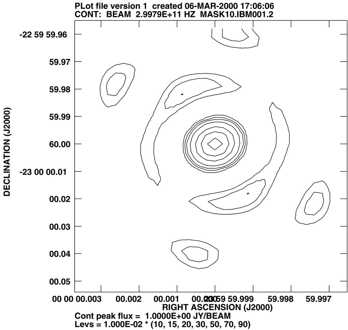
Figure 8: Snapshot observations. Beam pattern of the array fitted to the terrain using topography and doughnut constraints. The field ( $32 \times 32$ , cell =  $0.2 \frac{\lambda}{D}$ ,  $\lambda = 1mm$ ) includes only nearest side lobes. The side lobe level is about 20 %.
