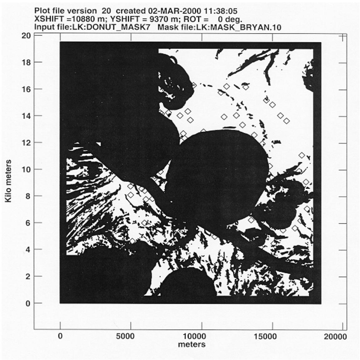
Figure 1: Array superimposed on 10 degree local gradient mask. The configuration is obtained optimizing side lobes with the topography as the only constraint.
