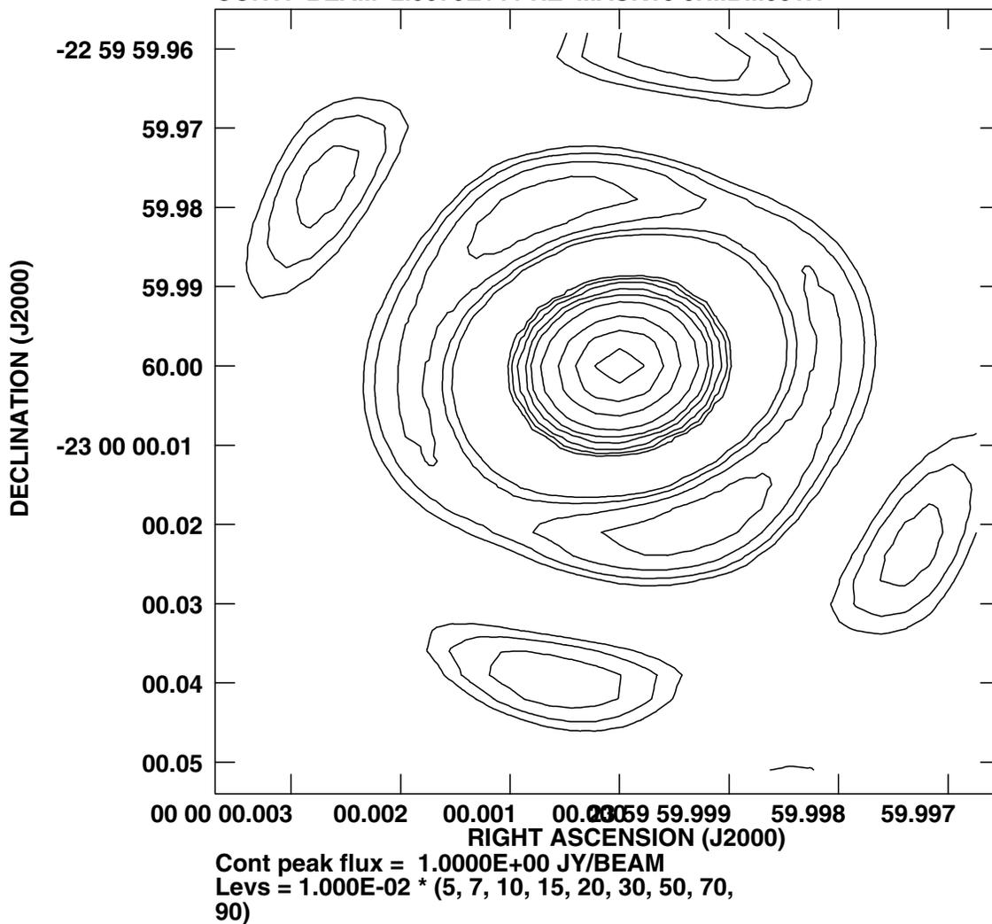
Figure 11: Six hour tracks observations. Beam pattern of the array fitted to the terrain using topography and doughnut constraints. The field ( $32 \times 32$ , cell =  $0.2 \frac{\lambda}{D}$ ,  $\lambda = 1mm$ ) includes only nearest side lobes. The side lobe level is about 17 %.
