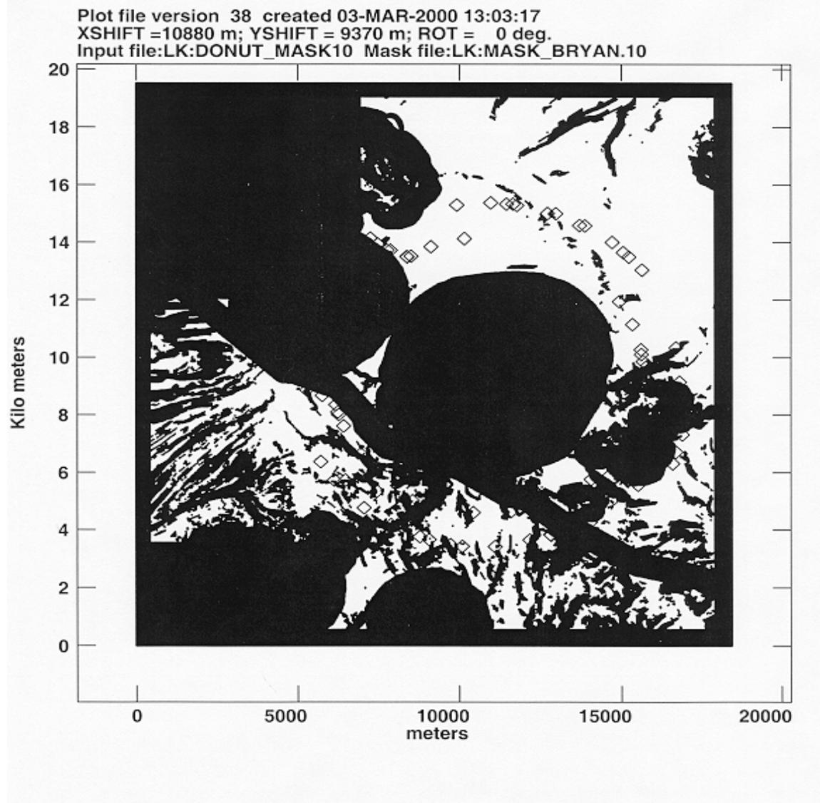
Figure 2: Array superimposed on 10 degree local gradient mask. The configuration is obtained optimizing side lobes with both the topography and the doughnut constraints.
