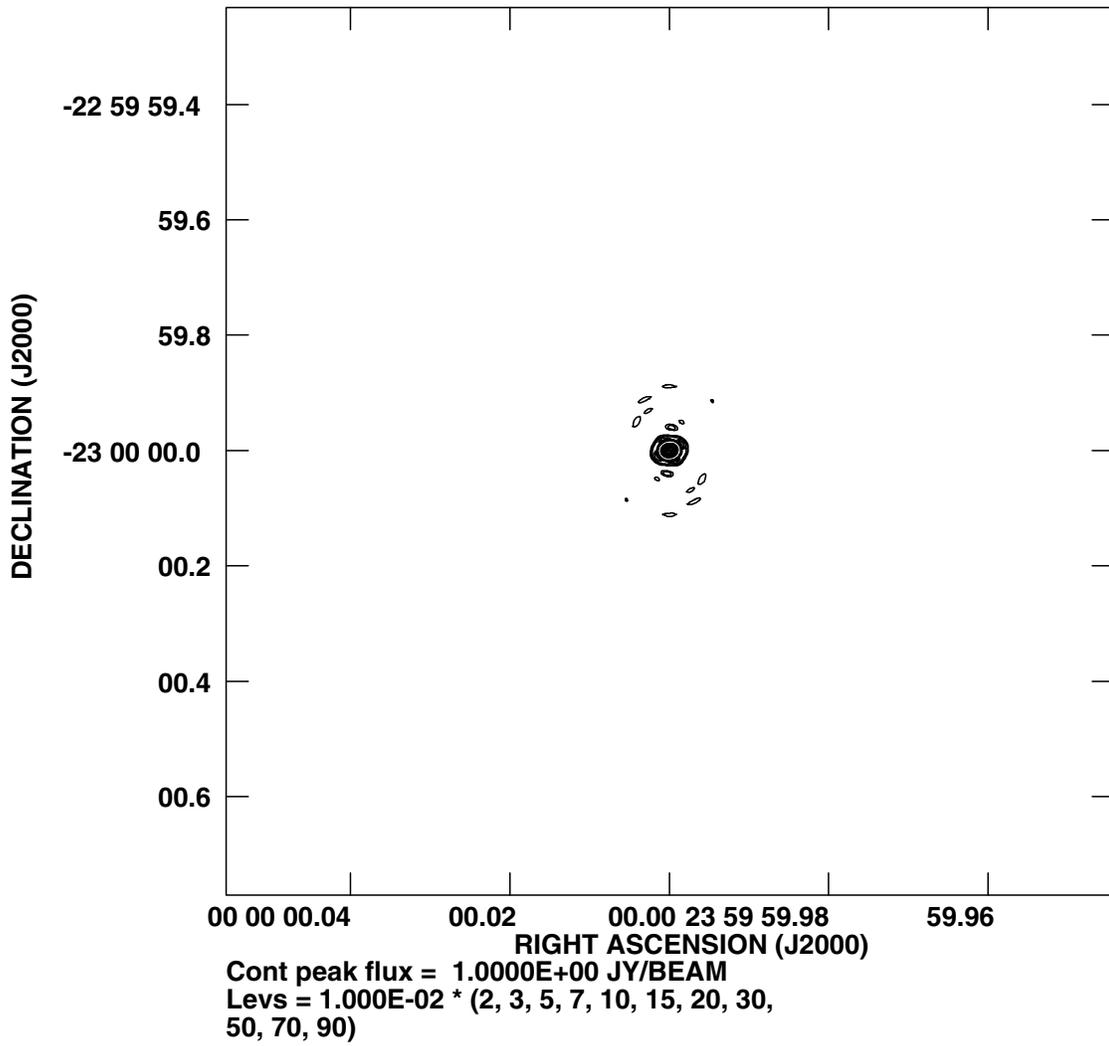
Figure 14: Six hour tracks observations. Beam pattern of the array fitted to the terrain using only topography constraints. The field ( $512 \times 512$ , cell =  $0.2 \frac{\lambda}{D}$ ,  $\lambda = 1mm$ ) includes far side lobes. UV coverage includes 6 hour tracks. The far side lobe level is less than 2 %.
