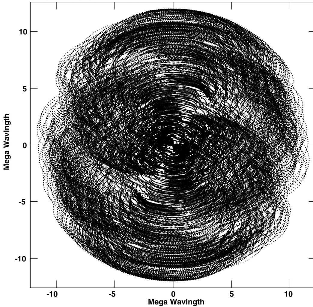
Figure 10: Six hour tracks observations. UV coverage of the array fitted to the terrain. The two constraints topography and doughnut were used at the fitting/optimization process. The AIPS task UVPLT used to create this file. Four visibilities of each five ones are skipped to diminish the size of the file. So actual UV coverage is more complete.
