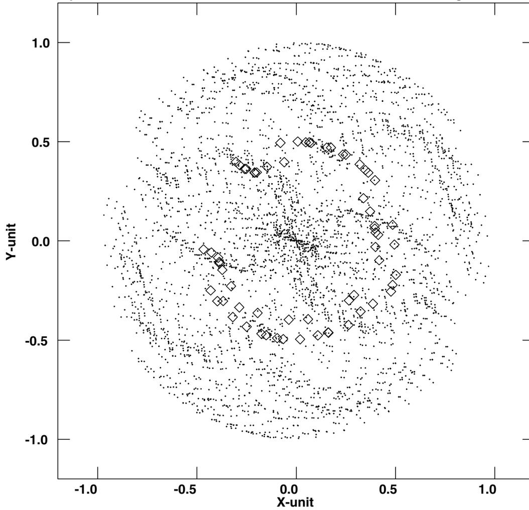
Figure 4: Configuration (diamonds) and snapshot UV coverage (dots) of the normalized array fitted to the terrain. The two constraints topography and doughnut were used at the fitting/optimization process. Size of the array is 12 kilometers.
