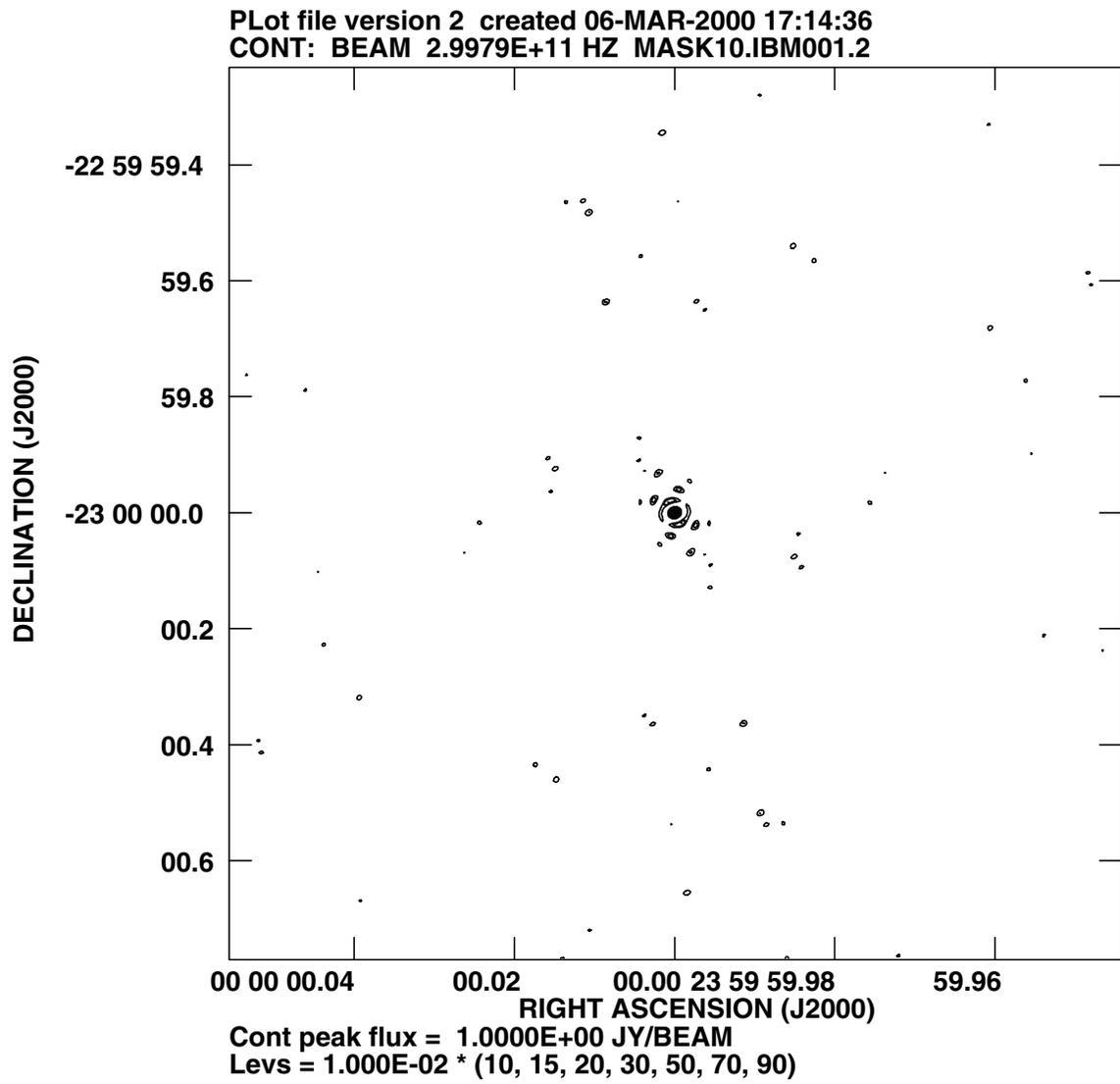
Figure 7: Snapshot observations. Beam pattern of the array fitted to the terrain using topography and doughnut constraints. The field ( $512 \times 512$ , cell =  $0.2 \frac{\lambda}{D}$ ,  $\lambda = 1mm$ ) includes far side lobes. The side lobe level is about 20 %.
