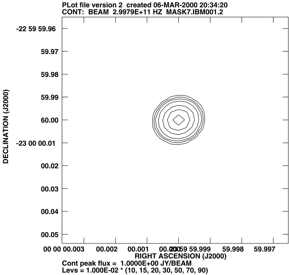
Figure 6: Snapshot observations. Beam pattern of the array fitted to the terrain using only topography constraints. The field ( $32 \times 32$ , cell =  $0.2 \frac{\lambda}{D}$ ,  $\lambda = 1mm$ ) includes only nearest side lobes. The side lobe level is about 10 %.
