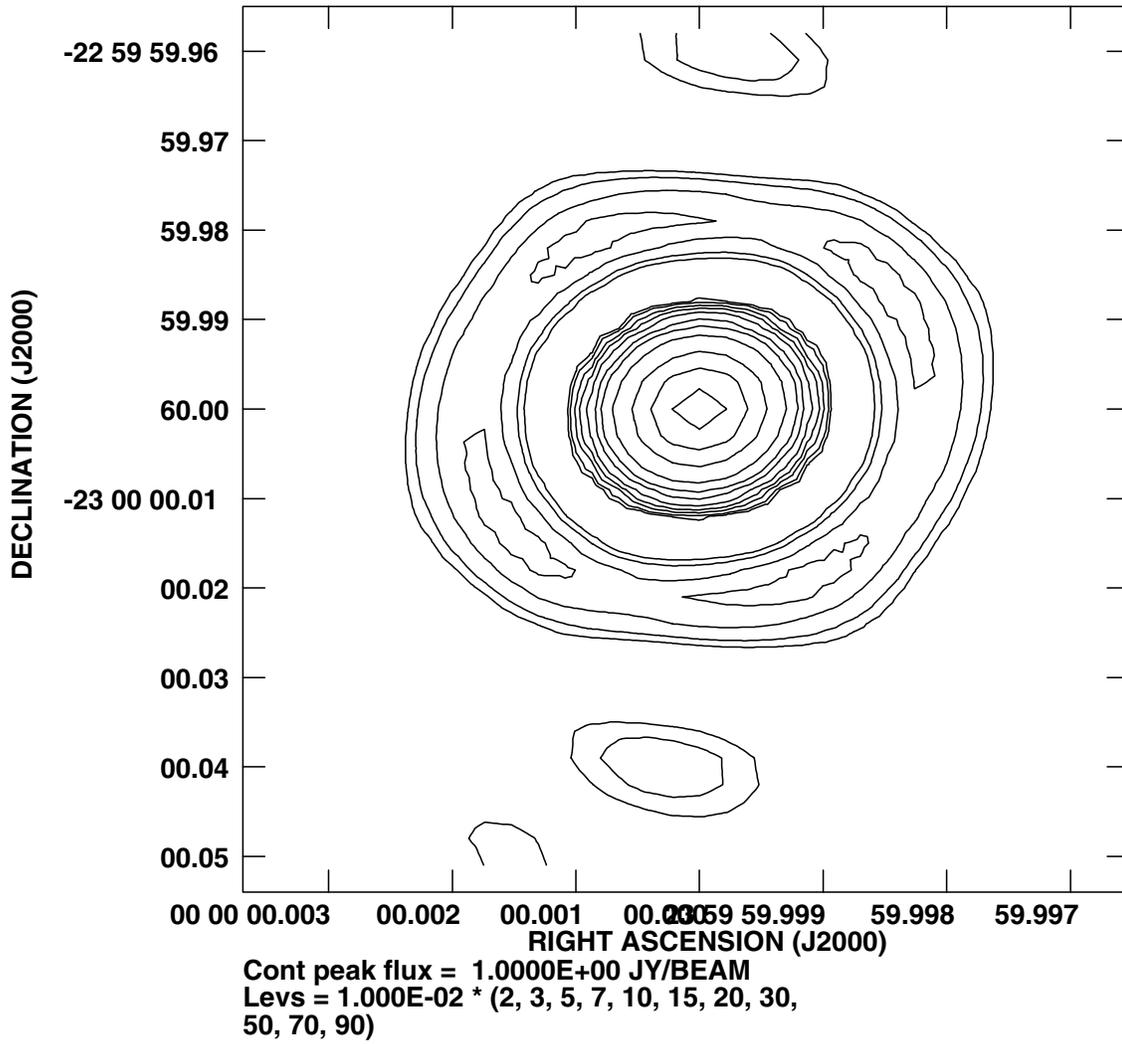
Figure 13: Six hour tracks observations. Beam pattern of the array fitted to the terrain using only topography constraints. The field ( $32 \times 32$ , cell =  $0.2 \frac{\lambda}{D}$ ,  $\lambda = 1mm$ ) includes only nearest side lobes. The side lobe level is about 8 %.
