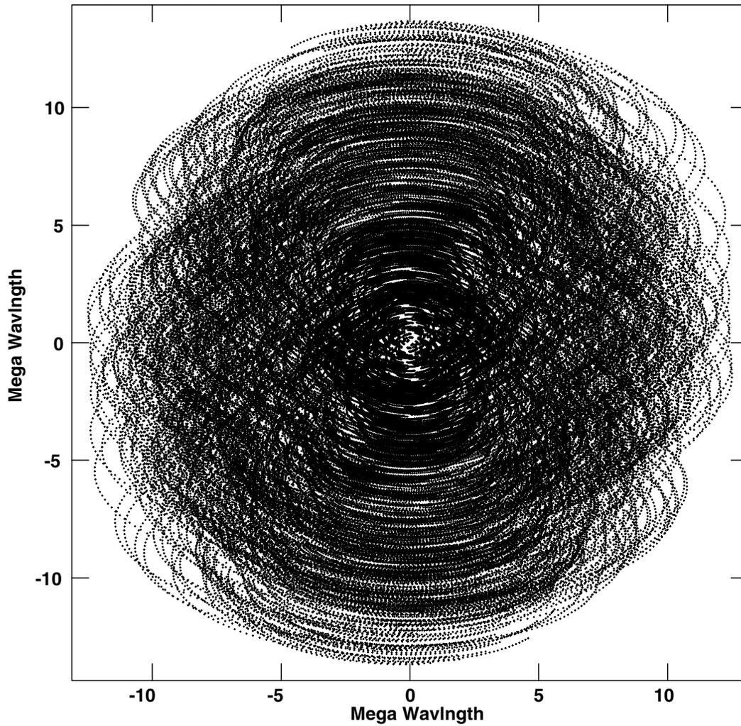
Figure 9: Six hour tracks observations. UV coverage of the array fitted to the terrain. The topography is the only constraint used at the fitting/optimization process. The AIPS task UVPLT used to create this file. Four visibilities of each five ones are skipped to diminish the size of the file. So actual UV coverage is more complete.
