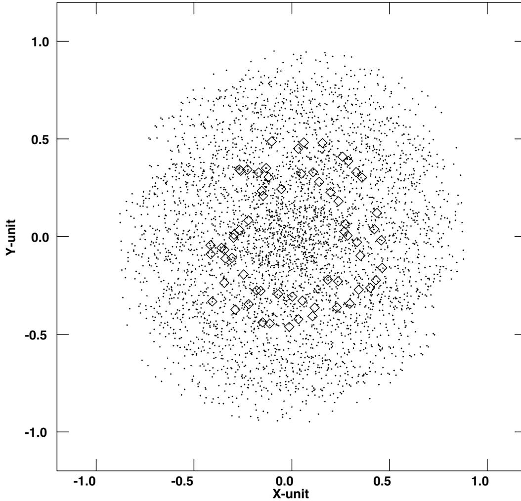
Figure 3: Configuration (diamonds) and snapshot UV coverage (dots) of the normalized array fitted to the terrain. The topography is the only constraint of the fitting/optimization. Size of the array is 12 kilometers.
