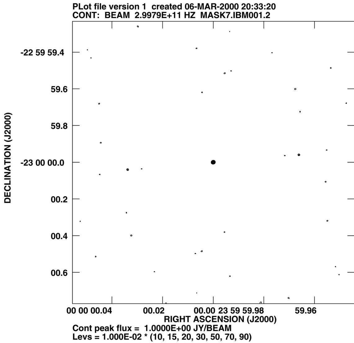
Figure 5: Snapshot observations. Beam pattern of the array fitted to the terrain using only topography constraints. The field ( $512 \times 512$ , cell =  $0.2 \frac{\lambda}{D}$ ,  $\lambda = 1mm$ ) includes far side lobes. The side lobe level is about 10 %.
