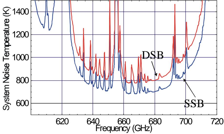
Fig. 5 The system noise temperature of a DSB receiver with mixer noise  $T_{SSB} = 300$  K and -10 dB LO coupling at 300 K compared with SSB receiver with mixer noise  $T_{SSB} = 300$  K, side-band separation of -10 dB, an -10 dB LO coupling and 60 K image dump black body temperature, 0.5 mm relative humidity.
