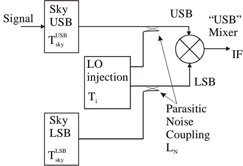
Fig. 4 Noise/Signal diagram of proposed receiver module. Only the USB mixer is shown.
