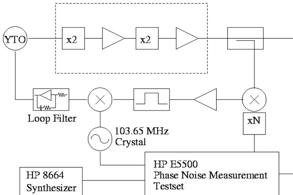
**Figure 1** Block diagram of phase noise measurement setup.
