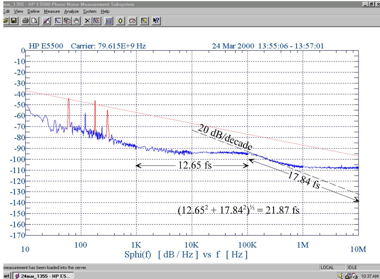
**Figure 6** HP E5500 phase noise measurement of 79.615 GHz YTO driver LO chain.
