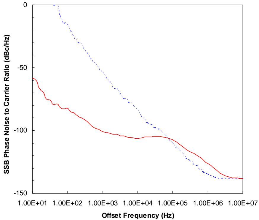
**Figure 2** Measured phase noise of the unlocked YTO (dashed line) at 21.0 GHz and the phase-locked YTO (solid line) at 20.9635 GHz.
