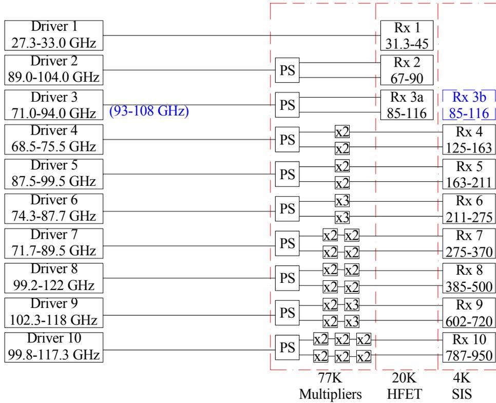
**Figure 8** Block diagram of proposed LO distribution plan.
