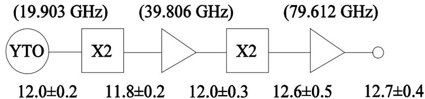
**Figure 5** Measured phase noise in femtoseconds integrated from 1-100 kHz at each point in the YTO driver chain. The uncertainty range is three standards of deviation.
