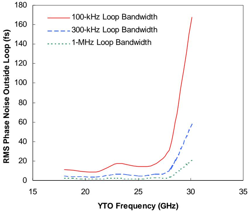
**Figure 4** Calculated rms phase noise integrated from loop cutoff to infinity for 100-kHz, 300-kHz, and 1-MHz loop bandwidths.
