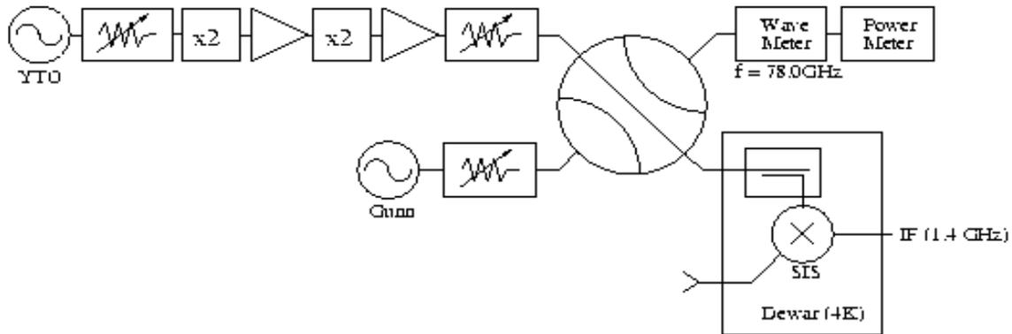
**Figure 7** Measurement setup for amplitude noise comparison of Gunn oscillator LO versus YTO driver LO.
