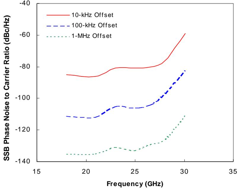
**Figure 3** Measured phase noise of the YTO at 10-kHz, 100-kHz, and 1-MHz offsets as a function of oscillation frequencies.
