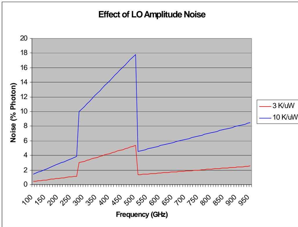
**Figure 7** The contribution of LO amplitude noise to receiver noise as a function of frequency. LO amplitude noise is given as percentage of a single photon for LO noise-to-signal  $(N/S)_{LO}$  values of 3 and 10  $K/\mu W$ . Balanced mixers with 10 dB LO noise rejection are assumed below 275 GHz.
