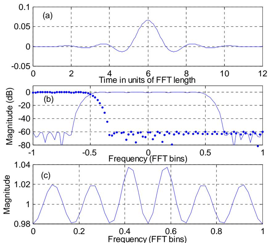
**Figure 3 Prototype filter and the response of the DFT filterbank it implements. (a) impulse response of prototype filter  $h_0(n)$ , (b) magnitude response of one of the outputs, response of adjacent output dotted and (c) sum of the correlation power for the two responses shown in (b)**
