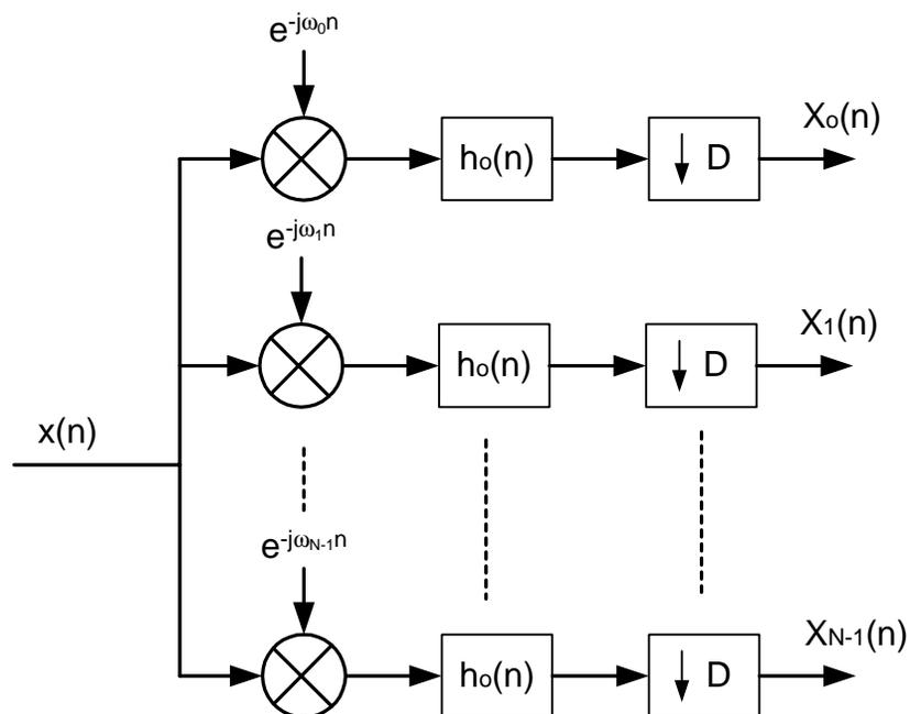
**Figure 1 Standard filter bank**
