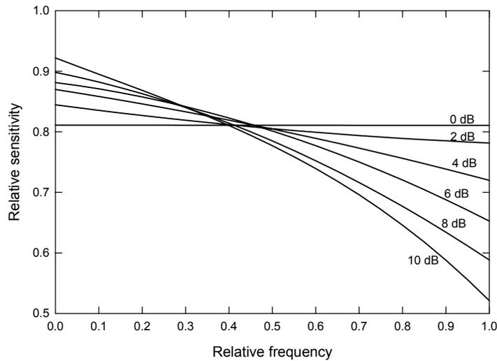
**Fig. 2.** Sensitivity of a 3-level correlator relative to a perfect analog correlator for various slopes in gain across the input bandwidth.
