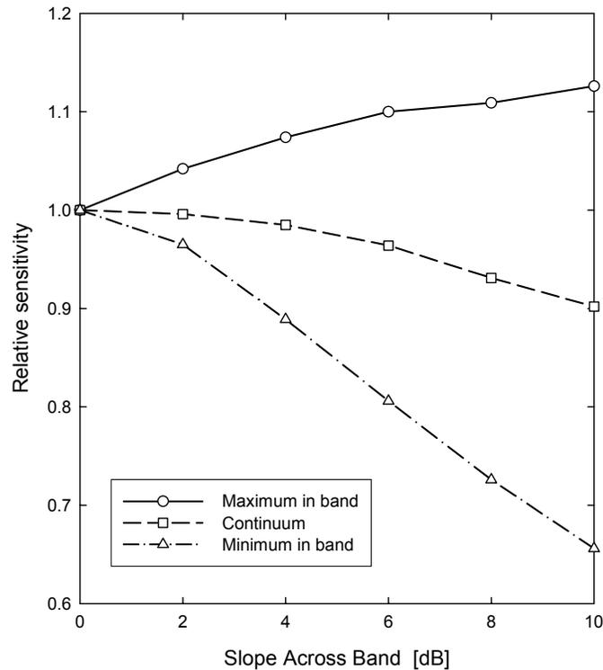
**Fig. 3.** Effective continuum sensitivity for a 3-level digitizer with various gain slopes across the band. The “maximum” and “minimum” correspond to the best and worst edges of the bands in the spectral mode, and the “continuum” corresponds to an optimally weighted sum of the channel measurements.
