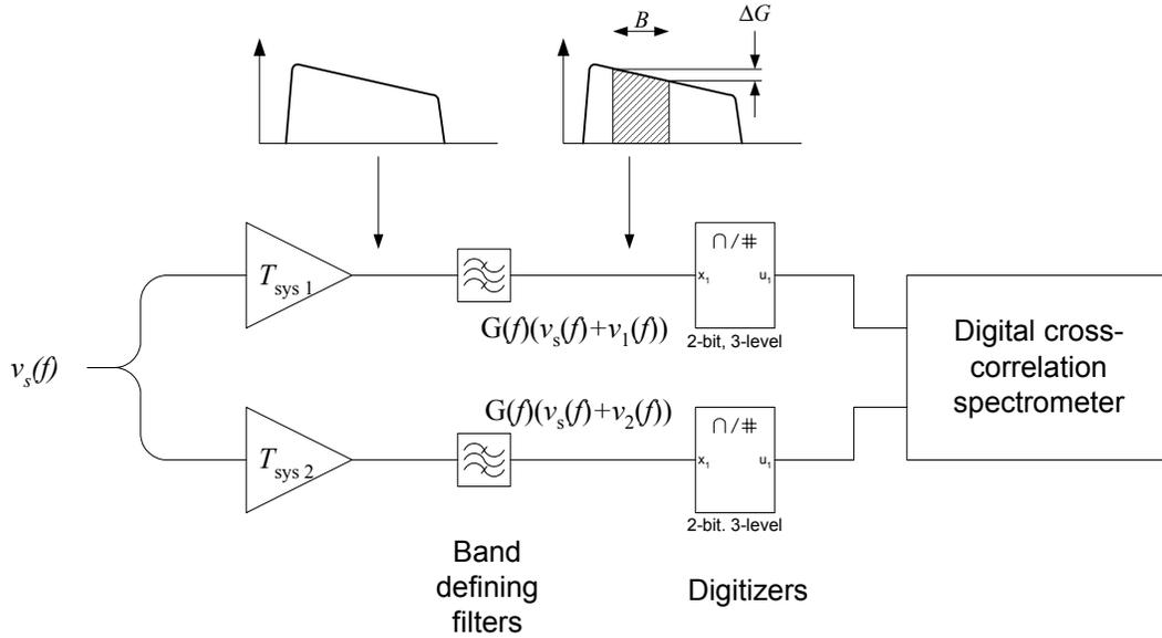
**Fig. 1.** A typical digital cross-correlator scheme. A correlated signal is sent into two paths with independent noise sources. The actual architecture of the digital part of the correlator is unimportant.
