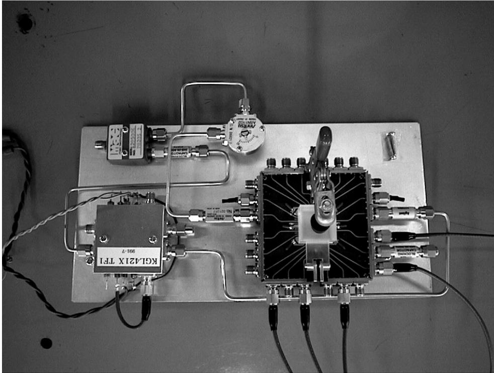
Fig. 3. Photograph of the 1-bit 8-Gbps digitizer circuit corresponding to the dotted square in Fig.2.
