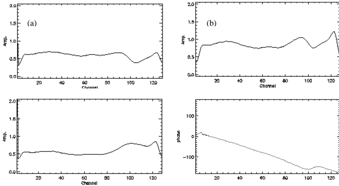
Fig. 4. (a) Amplitude spectra of the auto-correlation with 1-GHz bandwidth. Upper and lower spectra are for two AD Cs. (b) Spectra of the cross-correlation. The upper panel shows the amplitude spectrum, and the lower one shows the phase spectrum.
