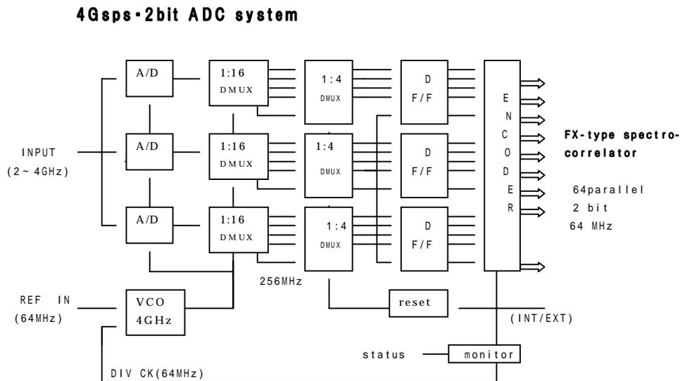
Fig. 6. Block diagram of 4-Gsps 2-bit ADC system using GaAs ICs. Shaded blocks are GaAs Decision and 1:16 DMUX chips, which have been confirmed their astronomical performances. Actually the encoder part is the separate frame from the other ADC part and they are connected with SCSI cables.
