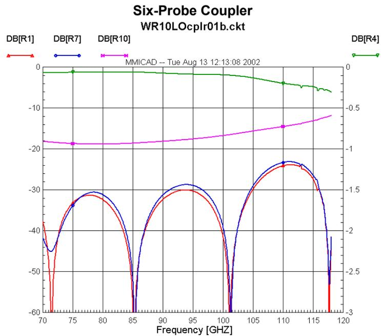
Fig. 6. Results of the QuickWave simulation of the six-probe coupler. Left scale: — S11 dB, — S31 dB, — S41 dB. Right scale: — S21 dB. (The WR-10 band is indicated by the markers at 75 and 110 GHz.)
