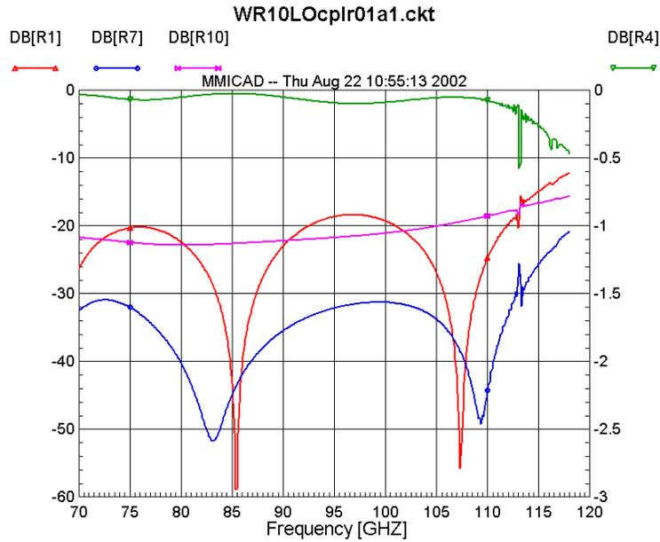
Fig. 7. Results of the QuickWave simulation of the four-probe coupler with all probes moved down 0.002". (Compare with Fig. 4.) Left scale: — S11 dB, — S31 dB, — S41 dB. Right scale: — S21 dB. (The WR-10 band is indicated by the markers at 75 and 110 GHz.)
