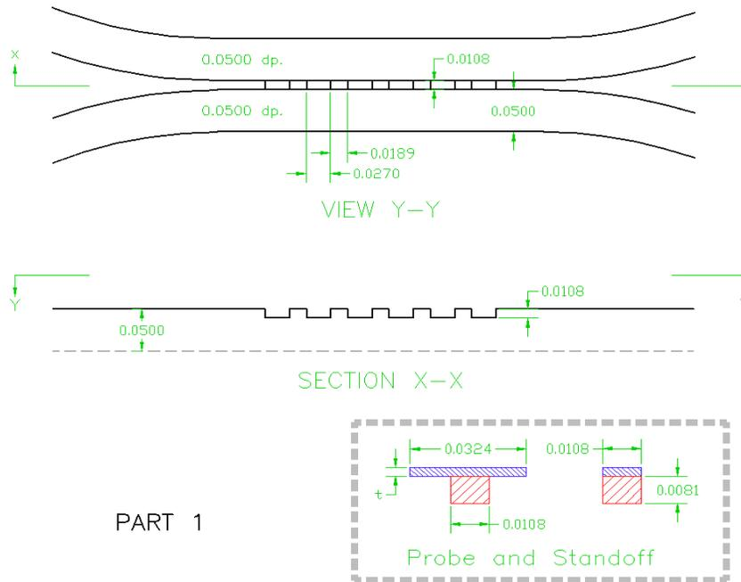
**Fig. 2. Dimensions of the WR-10 split-block coupler. Only the lower half-block is shown; the upper half is the mirror image. The box gives details of the probes (blue) and quartz standoffs (red). Dimensions are in inches. For the couplers tested below, the probe thickness  $t = 0.0016$ ".**
