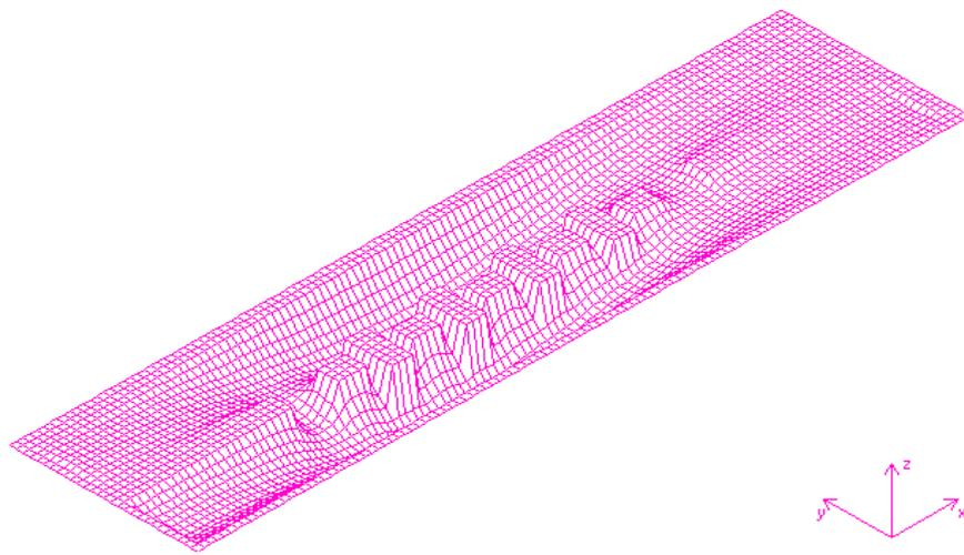
**Fig. 9. QuickWave simulation of the electric field component  $E_z$  in the four-probe coupler after the propagating components have died away. This trapped mode is weakly coupled to the dominant modes in the two waveguides and accounts for the small spikes seen just above the nominal waveguide band in the frequency characteristics of the coupler.**
