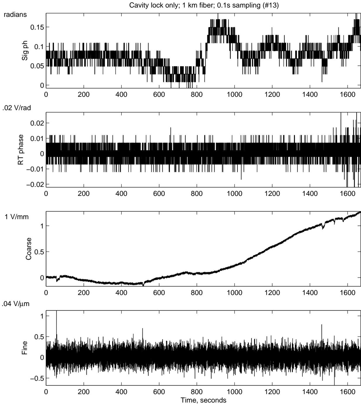
**Figure 6:** Similar to Fig. 5, but with 1 km of fiber and with the master laser locked to its optical cavity but not to the acetylene cell. It is believed that nearly all of the signal phase variation (704 fsec or 148  $\mu\text{m}$  p-p) results from frequency drift of the laser, but the length correction applied by the coarse stretcher is about 10 times larger and this is easily explained by length variation of the fiber due to a small temperature change.
