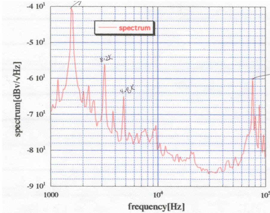
**Figure 7:** Spectrum of residual round-trip phase error obtained from dynamic signal analyzer. The UEC laser is used, locked to the C2H2 line and the external fiber length is 180m. The scaling is 250 mV/radian. The effect of the 1.6 kHz modulation and its harmonics at 3.2 and 4.8 kHz are clearly visible, as is the 75 kHz modulation due to a low-level oscillation in the laser-to-cavity locking loop.
