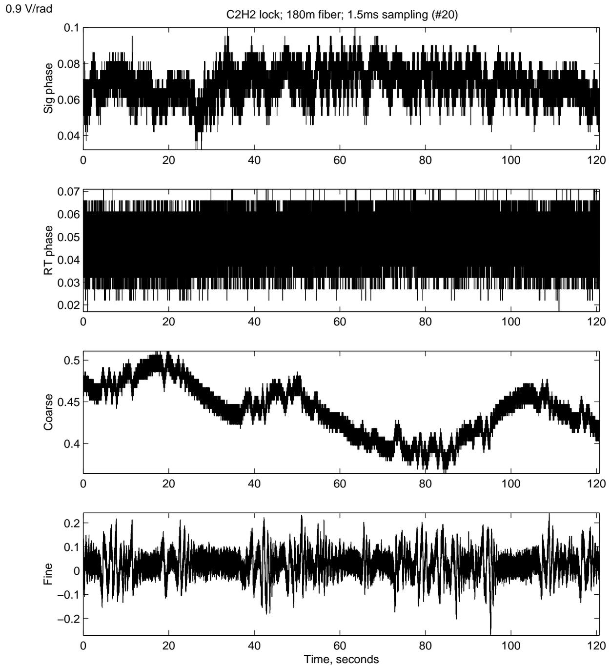
**Figure 8:** High time resolution measurement, with sampling period 1.5 msec. UEC laser locked to C2H2 line, 180m of external fiber. Features in the fine correction voltage may be vibration responses, perhaps to accidental disturbances. The following figures analyze this data in more detail.
