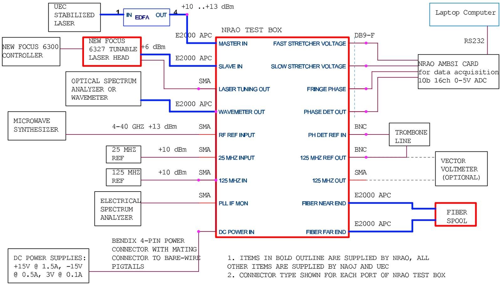
**Figure 2:** Test setup details, showing interconnections among devices.
