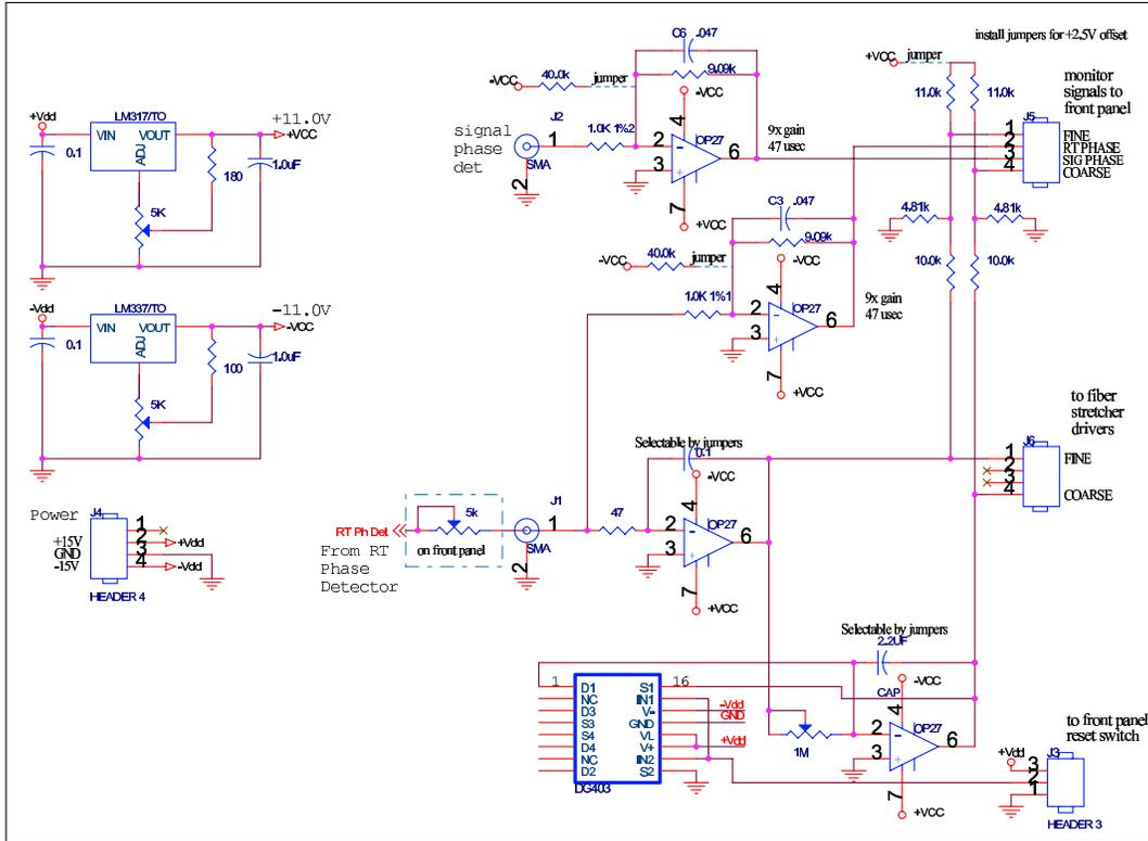
Figure 4: Schematic of controller board for correction loop, including filter/amplifiers for monitoring phase detector signals.
