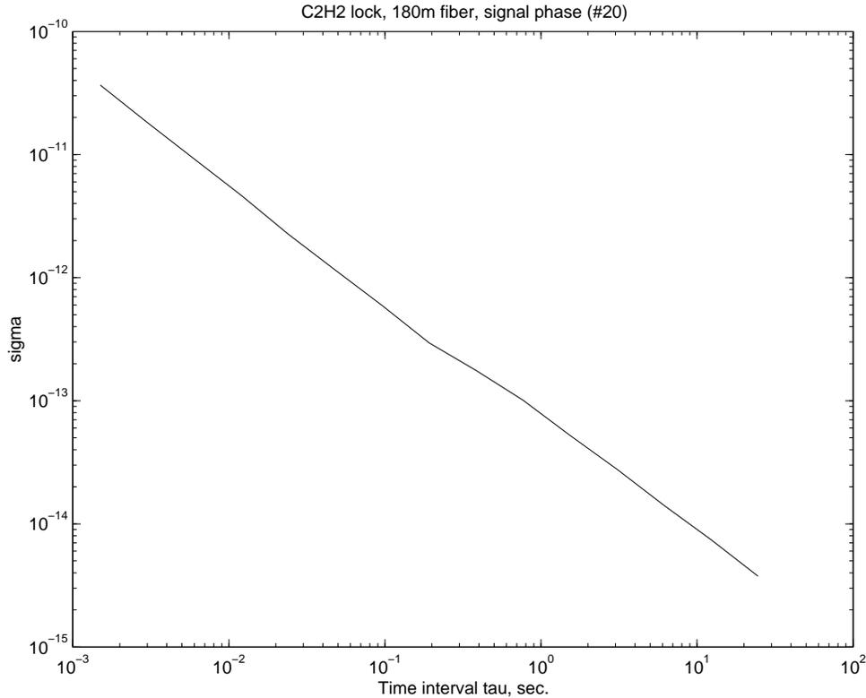
**Figure 10:** Allan standard deviation of the signal phase data from Fig. 8 at a frequency of 26.625 GHz.
