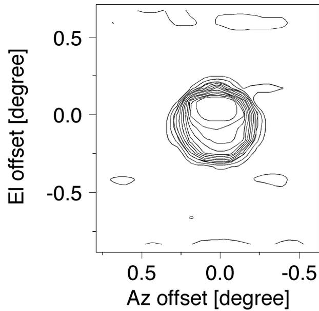
**Fig. 9.** First light of the moon with the band 10 receiver (LO frequency = 812 GHz). Age of the moon was about 12.4 days on 18 November 2002.
