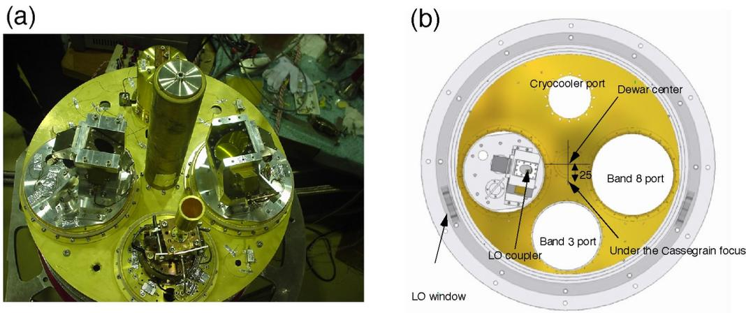
**Fig. 4.** (a) A photograph of the cryostat. 3 cartridge-type receivers (from right to left, 800 GHz, 100 GHz, 500 GHz) are installed. (b) A schematic drawing seen from the top of receiver system. The optical axis is inclined to the subreflector.
