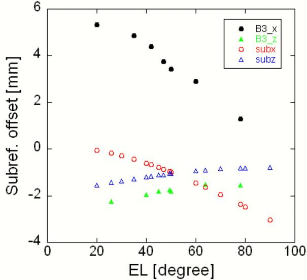
**Fig. 10.** Elevation dependence of optimum subreflector positions. The X and Z axis are vertical and focal offsets of the subreflector. Filled circles show best-fitted X-position of the subreflector measured by the band 3 receiver. Open circles show X position of the subreflector by a simulation. Triangles are the same as that of circles but for the Z axis. The relative difference between the measurements and the simulation can be explained by gravitational deformation of the band 3 receiver.
