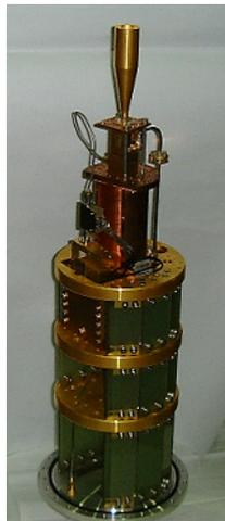
**Fig. 5.** A photograph of an engineering model of band 3 receiver.
