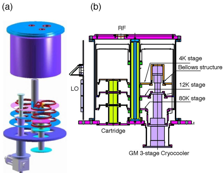
**Fig. 1.** (a) A schematic drawing of a cryogenic system for the ASTE, which houses 3 cartridge-type receivers. (b) A cross-sectional view of the cryostat. The cryostat is composed of 3 stages (from up to down 4 K, 12 K, and 80 K stage).
