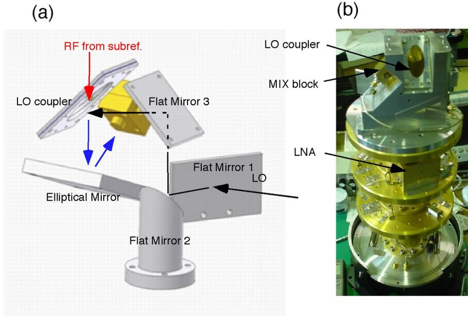
**Fig. 3.** (a) A schematic drawing of optics of band 10 receiver. (b) A photograph of the band 10 receiver. The RF optics consists of one elliptical mirror. The LO signal, which is introduced from the outside of vacuum vessel, is coupled quasi-optically to the RF signal by the dielectric, Kapton. The coupling factor of LO is -10 dB. The LNA with a gain of 35 dB is attached on the 12 K stage.
