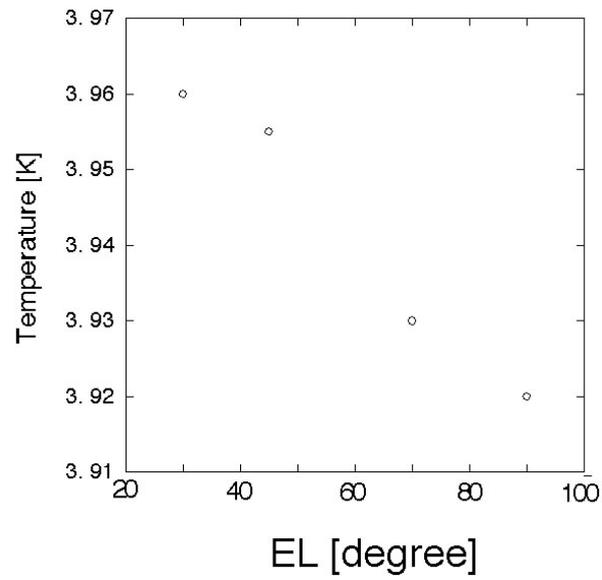
**Fig. 8.** Elevation dependence of temperature on the 4 K stage of the band 8 cartridge. A difference of temperature between at 90 degree and at 30 degree was about 40 mK.
