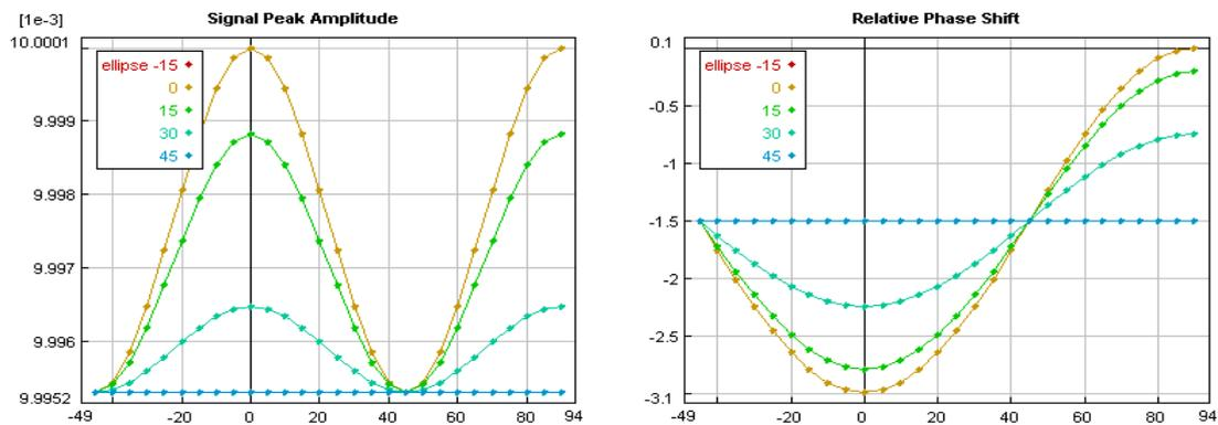
Figure 5 RF signal amplitude and phase change for a 100 GHz signal when the input SOP rotates.
