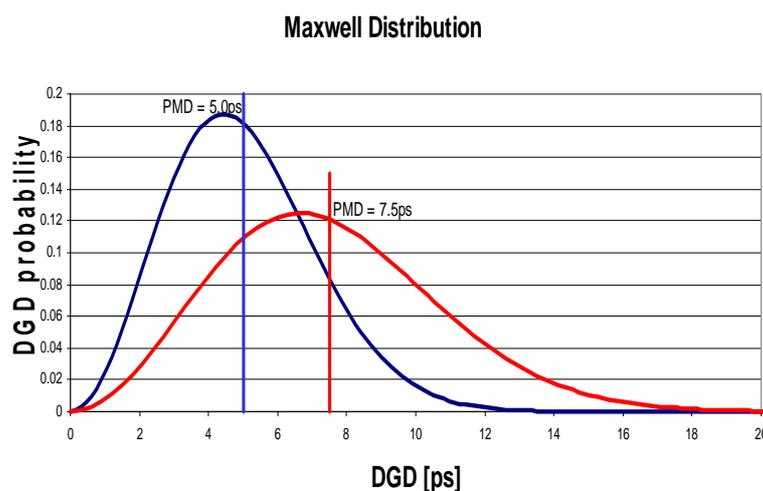
Figure 1 Typical DGD distribution of a long fibre at a fixed  $\lambda$  for two values of PMD. The mean of each distribution is shown by a vertical line, which defines the PMD value.
