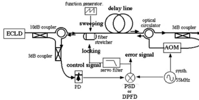
**Figure.3:** Schematic diagram of the fiber length stabilization system (FLSS). The fiber length can be swept by applying saw-tooth signal to the fiber stretcher, and the stabilization loop is closed when the control signal is applied to the fiber stretcher.
