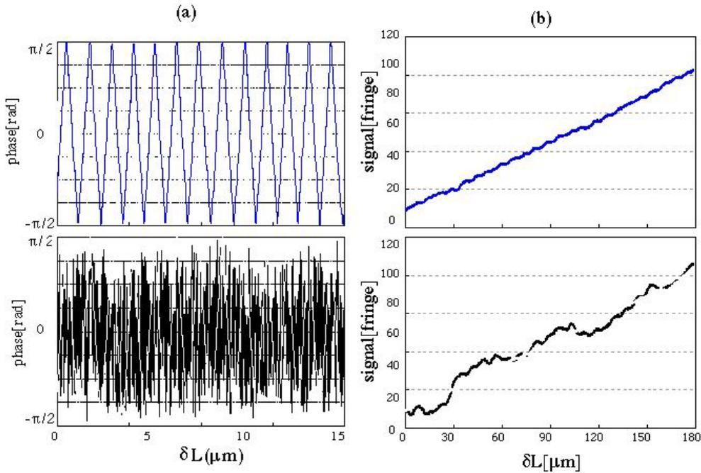
**Figure 4:** The error signals from (a) PSD and (b) DPDF. In both figures, the length of the fiber is 10m (upper case) and 25km(lower case).
