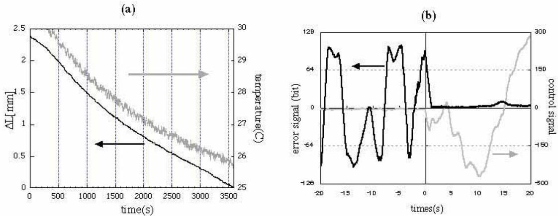
**Figure 5:** (a) The temporal behaviors of the fiber length fluctuation, which is calculated from the control signal (black trace), and the temperature of the fiber (gray trace). (b) The error (black) and control (gray) signal of the length correction servo at the fiber length of 25 km.
