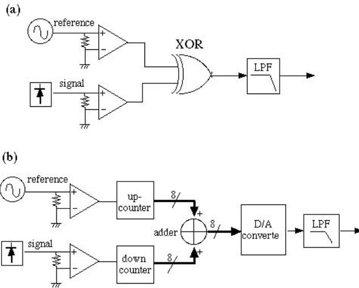
**Figure.1:** Schematic diagram of (a) conventional digital PSD and (b) digital phase and frequency discriminator (DPFD)
