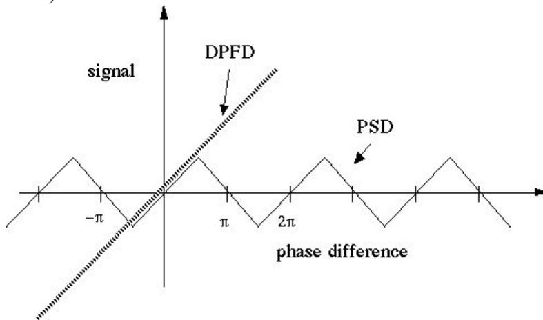
**Figure.2:** The phase error signals from PSD (solid trace) and DPF (dotted trace)
