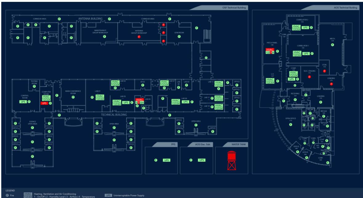
Figure 7 - Display of OSF and AOS buildings showing real location of HVAC systems, fire alarms and other supplies
