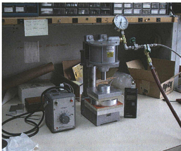
From left to right: Variac, air press, press components, digital thermometer, pressure gage, press valve, vent-valve to air blow gun, hose to nitrogen bottle regulator.
