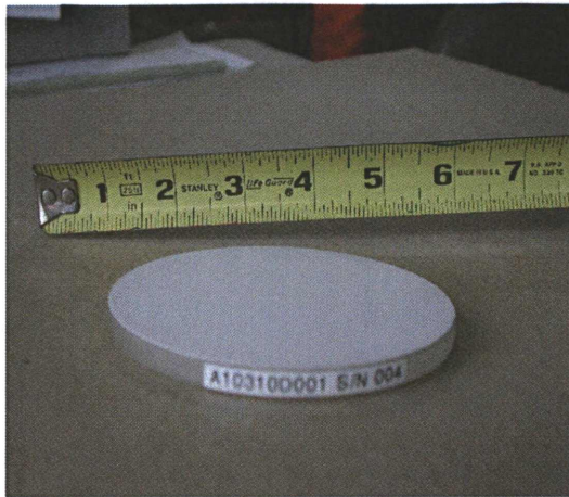
Finished 5 layer window, top side
