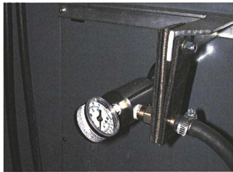
Lathe rotary coupler and vacuum gage
