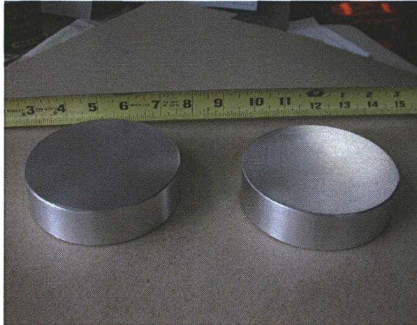
4" diameter epoxy transfer disks
