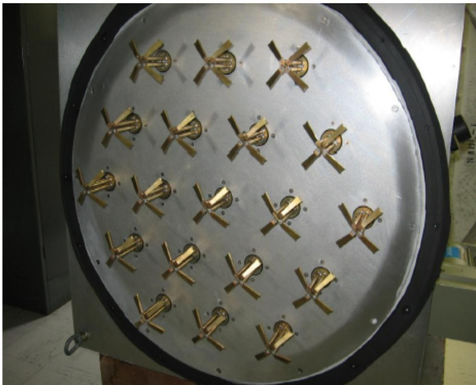
Figure 1: Image of “Kite” dipole is shown on the left and the 19 element dual-polarization “Kite” array on the right.
