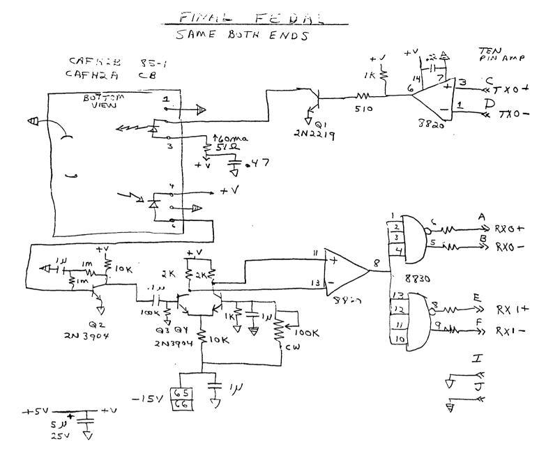
TXO+ nor Low - HIGH = 12% time Boud period = 50 ps at InterFormation link now. TXO+ high >Q1 on > 60 mi thru LED > cur thru Pin DioDE receiver -> Q2 col meg going > Q4 nor brased high goes negative > 8 of 8520 Low -> RXO+ High. 100K resistor adjusted to slice arout full to keep Boud period out T: Boud period lin - in This case 50 MS.
