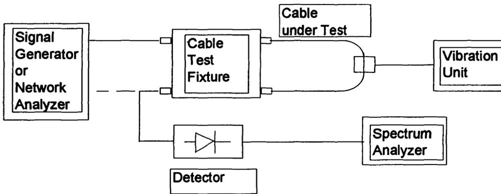
Figure 1. Test configuration for baseline, compression, tension, and vibration tests.
