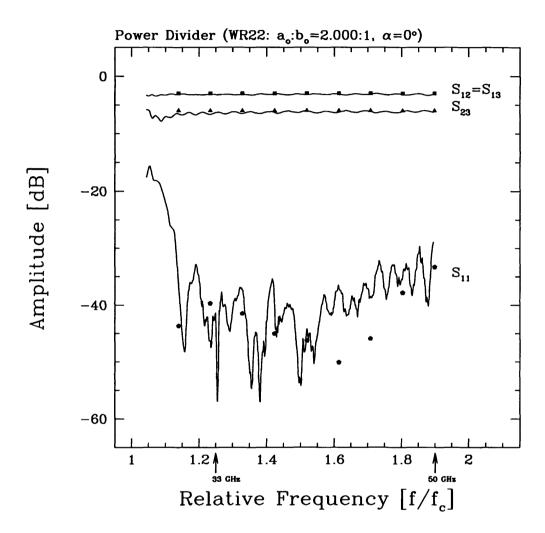
Figure 4. Measured Response: Bifrucated Waveguide "A" Power Divider (Septum;  $t/a_o = 0.05$ ,  $\alpha = 0^o$ ). The computed finite element response is indicated by solid points in the figure.
