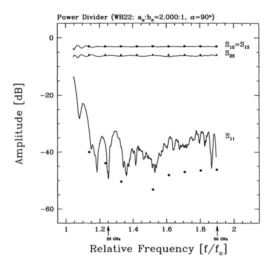
Figure 5. Measured Response: Bifrucated Waveguide "C" Power Divider (Mitre;  $\alpha = 90^{\circ}$ ). The computed finite element response is indicated by solid points in the figure.
