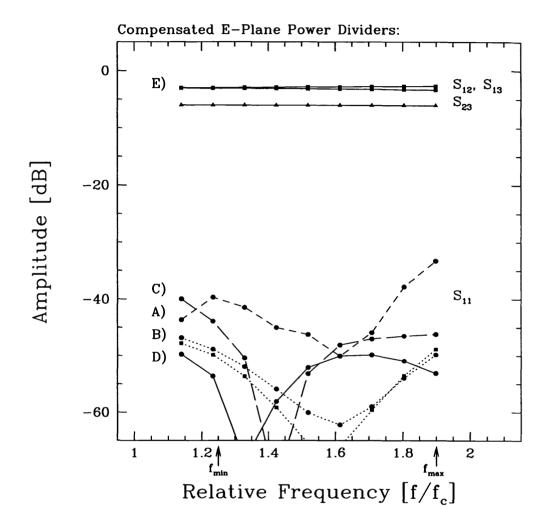
Figure 3. Selected Modeled Responses of Compensated E-Plane Power Divider Junctions: The asymmetry between  $S_{12}$  and  $S_{13}$  indicated in the figure is the worst case encountered (test case "E";  $\alpha_1 \neq \alpha_2$ ). Achievable designs with unequal power division,  $b_1 \neq b_2$ , result in discrepancies of similar magnitude from the design goal.
