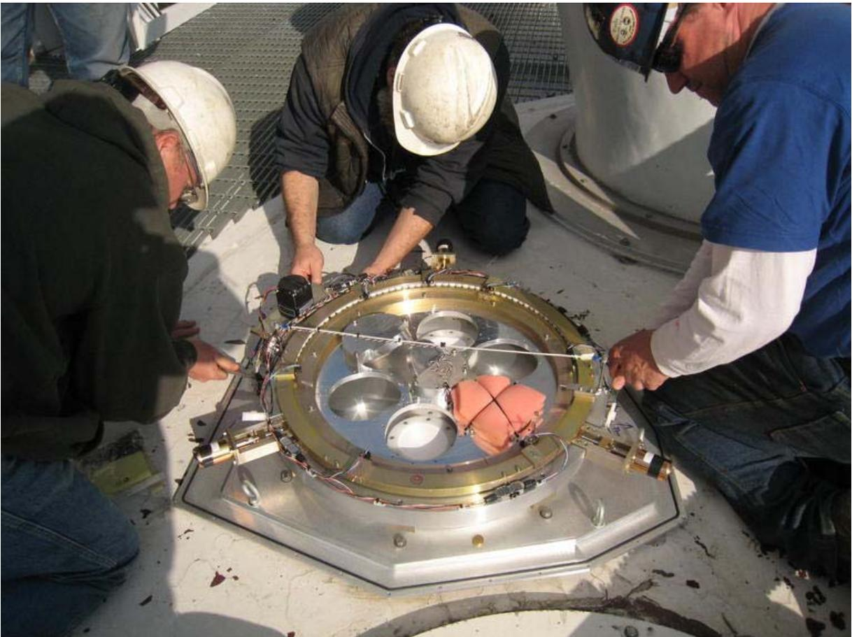
Figure 3. Photograph of the 4mm calibration wheel when mounted on the GBT turret. The position of the wheel, as shown, is two-pixel observing.
