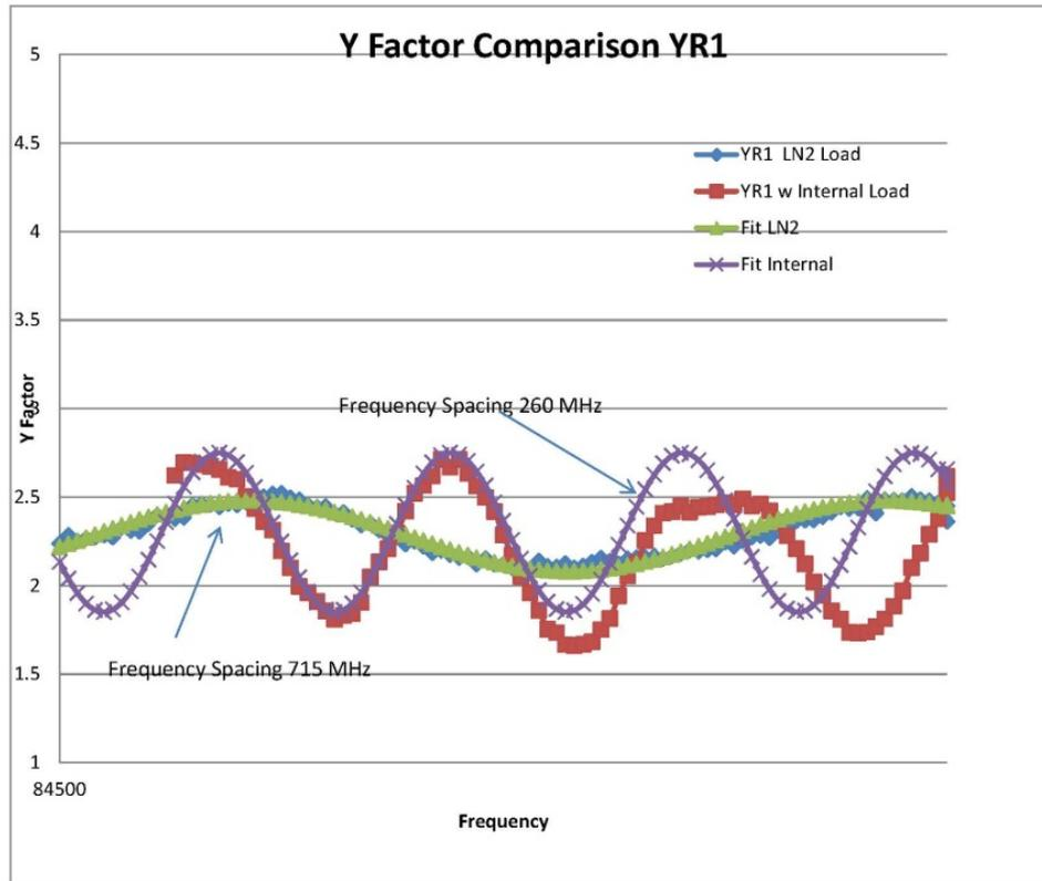
Figure 5. Comparison of Y-factors: internal cold load and external LN<sub>2</sub> load. The curve fit to the LN<sub>2</sub> load was in very good agreement with the reflected lengths of the cavity. The internal load indicates more than a simple reflection model is needed.
