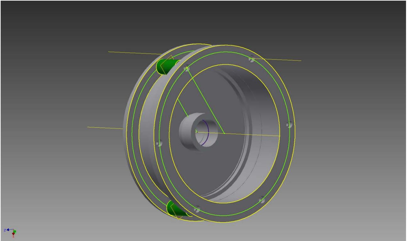
Figure 6. Shroud with thermal gap constructed around each feed that isolates the feed from the cavity. The cavity length is 1.1", and the diameter is 3.6".
