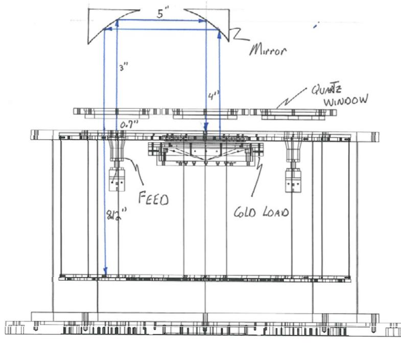
Figure 2. Path length of reflections from internal cold load to feed. Including the path to the bottom radiation shield, the total is 24.1".
