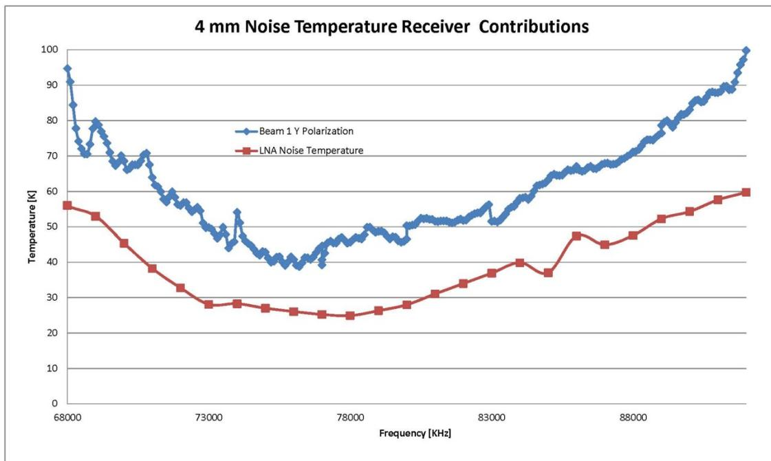
Figure 7. YR1 Noise temperature measurement illustrates improvement.
