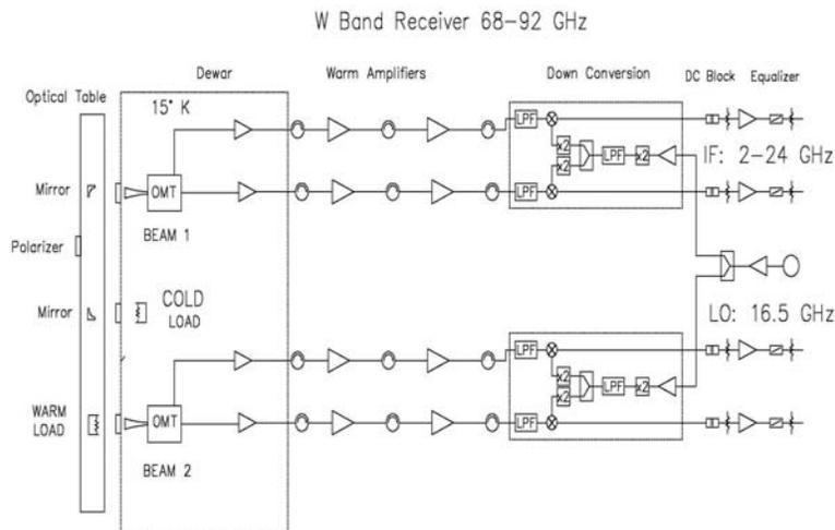
Figure 1. Receiver Block Diagram
