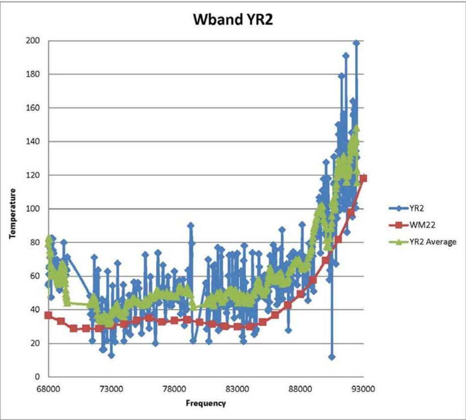
Figure 4. W-band channel YR2 noise temperature measurement.
