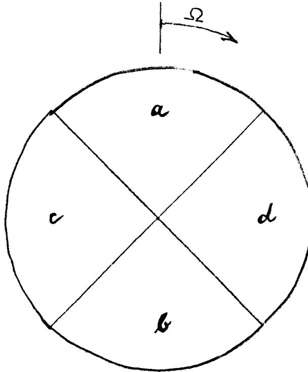
Fig. 1. The deformable subreflector, with two stiff diagonals, and four actuators pushing or pulling by amounts  $a$ ,  $b$ ,  $c$  and  $d$ . This yields four degrees of freedom for its use, to be called:
