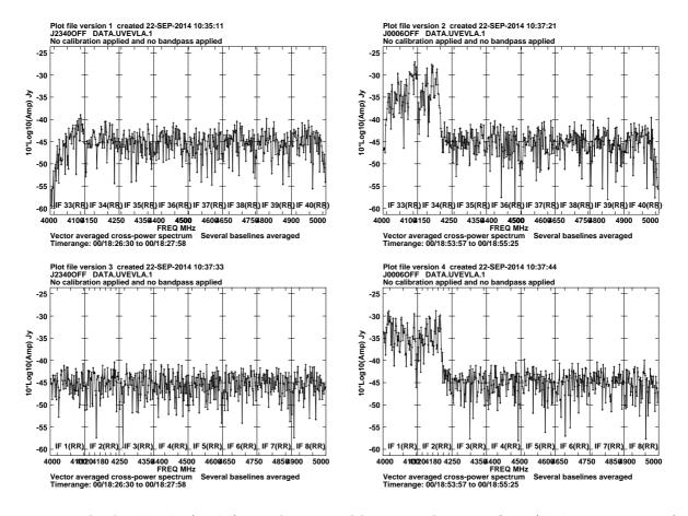
Figure 1: Left: Amplitude (in dB) as a function of frequency for J2340OFF (declination ~ +49°). Right: The same again for J0006OFF (declination ~  $-6^6\circ$ ). The Top panels display data from the 8-bit system and the Bottom panels display data from the 3-bit system. At declinations close to the satellite belt, the spectral flux density of the first two spectral windows is ~10 - 15 dB higher than the "RFI-clean" spectral windows.
