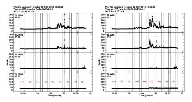
Figure 2: Left: System temperature vs UTC time for each spectral window from EA05 using the 8-bit samplers. Scan boundaries are shown as vertical lines. The declinations of the sources are marked in magenta on the lowest panel. Only the first four spectral windows are shown in each plot as the remaining spectral windows look similar to the bottom two spectral windows. Right: Same as left panel except using 3-bit samplers.
