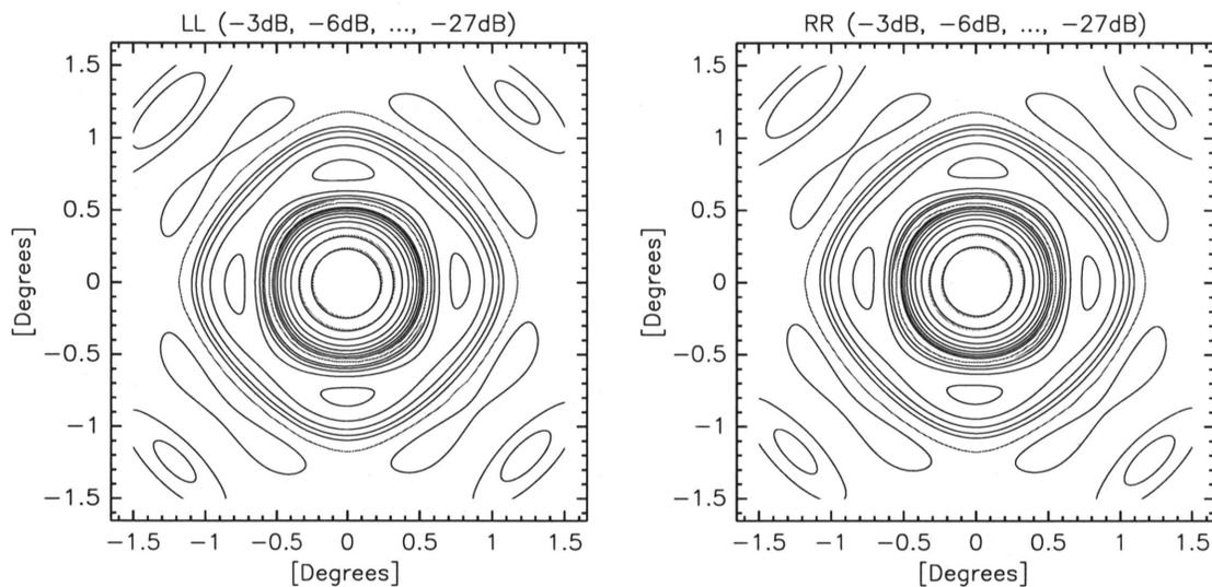
Figure 4: The VLA beam at 1.53 GHz in Left (LL= $I-V$ ) and Right (RR= $I+V$ ) polarizations. Superimposed on these plots are green contours showing the  $-3$  and  $-6\text{dB}$  total power contours and red contours showing the first two nulls. Note the beam squint that separates the LL and RR beams. The squint is more easily seen in the 1-D beam cuts of Figure 5. As for Figure 3, the Stokes  $V$  data were antisymmetrized before computing the LL and RR beams.
