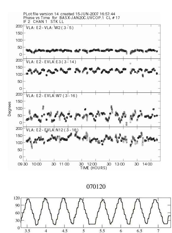
Figure 1a: Baseline data from January 20, 2007 showing phase variation after best-fit antenna positions have been removed (top) and corresponding antenna elevation (bottom).
