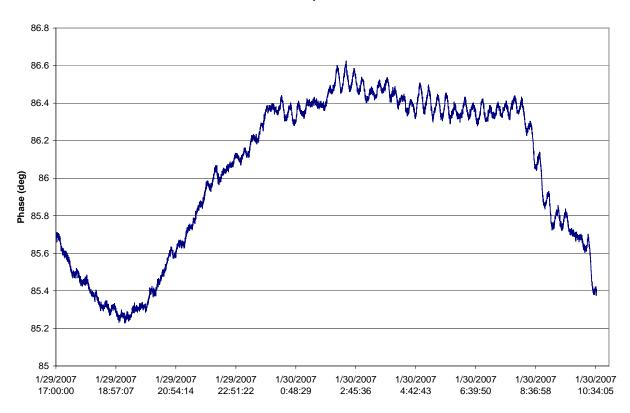
Figure 1d: Deformatter phase @ 50MHz, clocking DDS with recovered data clock. The sawtooth phase variation has a non-stationary frequency, and does not correlate to antenna tipping.
