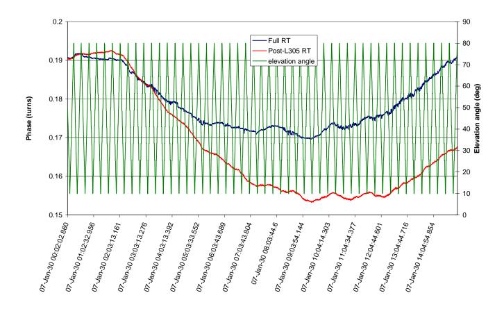
Figure 1c: Antenna 26 Round trip phase and antenna elevation angle. No elevation signature is present in round trip phase measurement.
