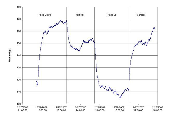
Figure 3a: Laboratory tip test. Phase of L300/L302/T304 system versus stationary reference signal. Tip points are clearly articulated.
