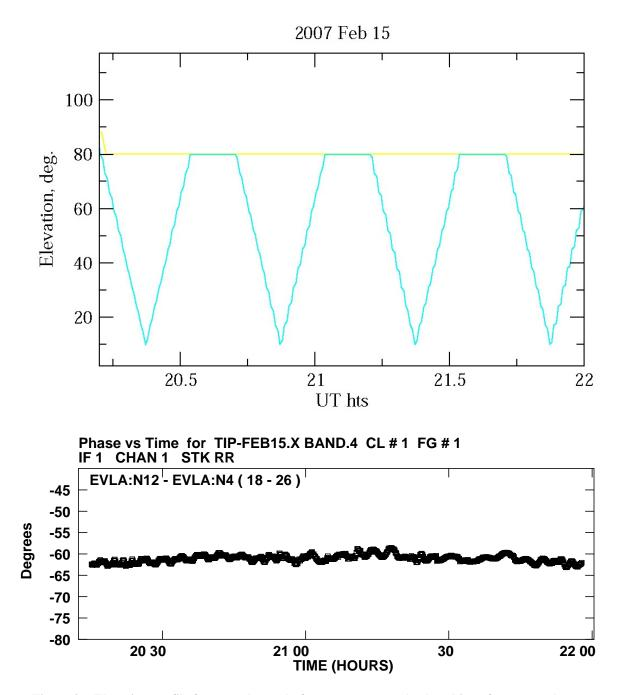
Figure 2a: Elevation profile for second round of on-antenna tests (top) and interferometer phase (bottom). The elevation signature is not present in the correlation of the injected signal.
