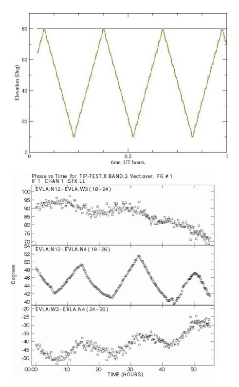
Figure 1b: Elevation profile (top) and phase of IF 1-L for the three baselines of injected CW signal on correlated signal (bottom). Elevation signature is clearly discernible in the 18 – 26 baseline.
