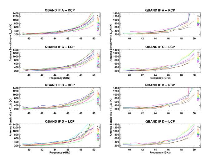
Figure 2: Q-band antenna sensitivities. EVLA antennas (left) and VLA antennas (right) for all IF's and polarizations.
