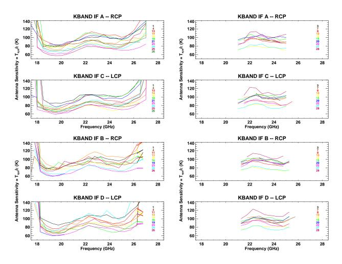
Figure 1: K-band antenna sensitivities. EVLA antennas (left) and VLA antennas (right) for all IF's and polarizations.
