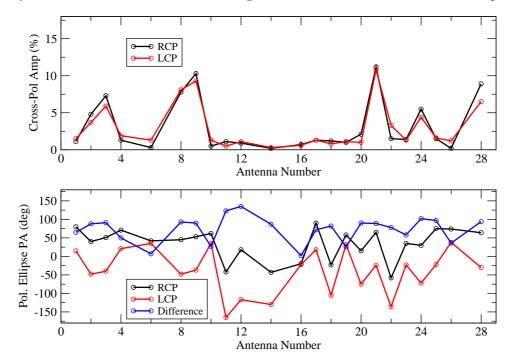
Figure 2: The same as in Fig. 1, but for 4885 MHz. The antennas equipped with the narrow-band VLA polarizers show excellent purity. The new wide-band polarizers (on antennas 3, 4, 8, 9, 21, 24 and 28) are notably less pure.
