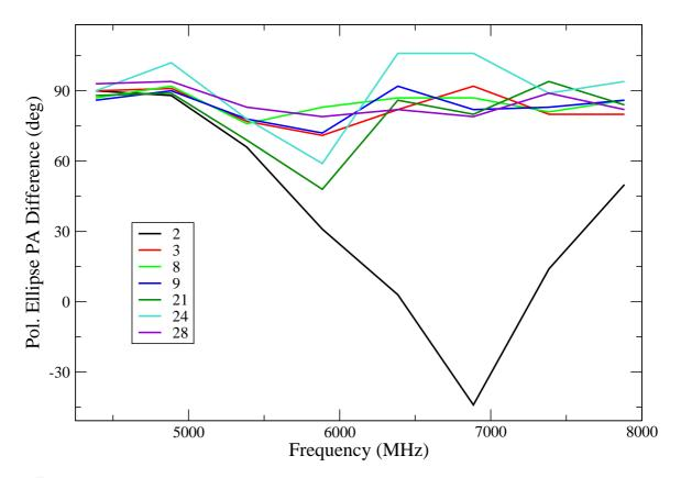
Figure 4: Showing the orthogonality of the EVLA antenna polarization ellipses. Except for antenna 2 (whose polarization at the higher frequencies is very low), the differences are close to 90 degrees, enabling acceptably low leakages in the cross-polarization baseline-based correlations.
