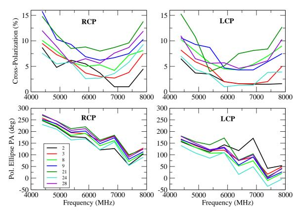
Figure 3: The upper panels shows the absolute cross-polarizations for all seven functioning EVLA antennas equipped with wide-band OMTs for RCP (left) and LCP (right). The lower panel shows the orientations of the polarization ellipses. The differences between RCP and LCP are close to 90 degrees for all antennas.
