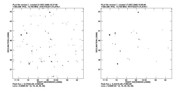
Figure 7: Comparison of the images for Cotton's data(4-band). The left plot is the image using UVAVG task (vector averaging in 360s). The right plot is the image using UVRFI. OPTYPE = 'CEXP'. Solution interval = 360s
