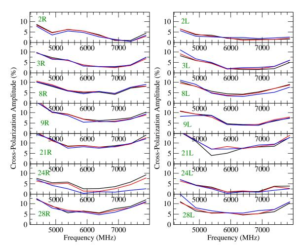
Figure 5: The change in C-Band cross-polarization for the seven antennas that have had wideband feeds since April 2009. The April 2009 results are shown in black, the January 2010 in red, and the new March 2011 in blue. For nearly all antennas, the change in cross-polarization over the two-year period is nor more than a few tenths of one percent.
