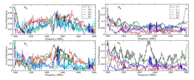
Figure 3: (Left) Cross-Polarization Amplitudes at L-band for five antennas outfitted with new design low-temperature quadrature hybrids. (Right) The results for five antennas with old-style. Note the change in scale. The new style provides better performance overall.
