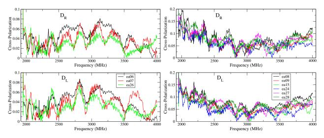
Figure 2: (Left) The cross-polarization amplitudes at S-band for three antennas outfitted with new design quadrature hybrids. (Right) The cross-polarization amplitudes for the old design hybrids. Note the change of scale – the old design is notably poorer than the new over the entire frequency range.
