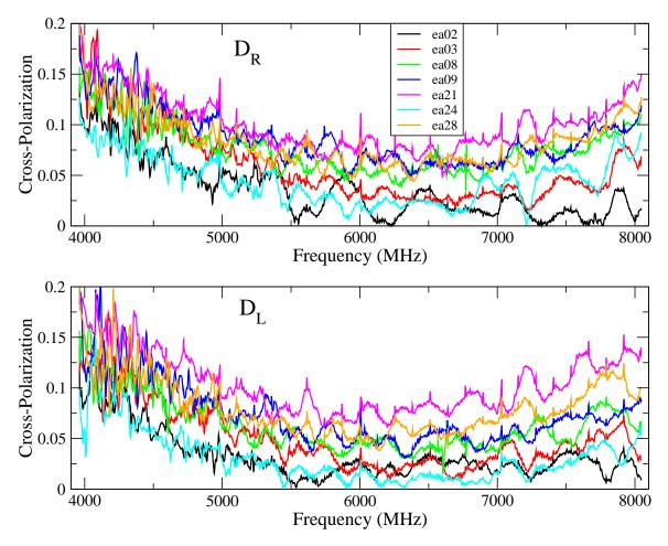
Figure 4: Cross-Polarization Amplitudes for seven antennas outfitted with the old quadrature hybrids at C-band.
