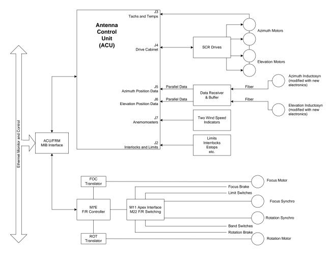
Figure 1 - Simplified Control System Block Diagram
