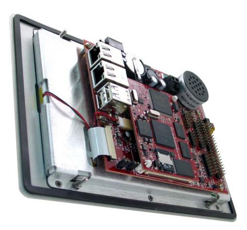
Figure 5 - Embedded Touch Panel Computer
