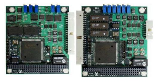
Figure 4 - PC-104 Processor and Peripherals
