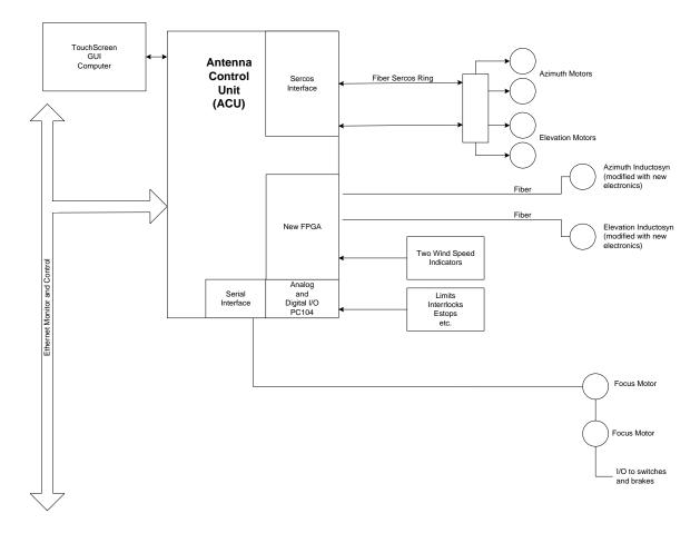
Figure 3 - Upgrade Maximizing Flexibility and Advantages of Up to Date Hardware
