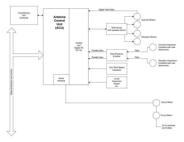
Figure 2 - Upgrade Reusing Current Drives and Sensors
