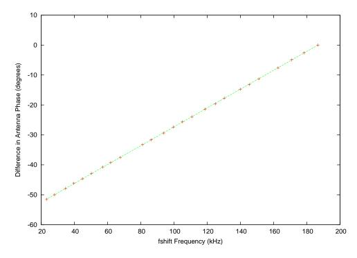
Figure 4: The phase difference in antenna gains, as a function of  $f_{\text{shift}}$ , with and without recirculation. The crosses are the measured difference whereas the line is the expected difference.
